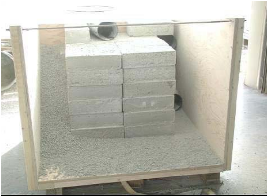
Figure 10: Light Backfill Pneumatic Emplacement Trials at AECL's URL
