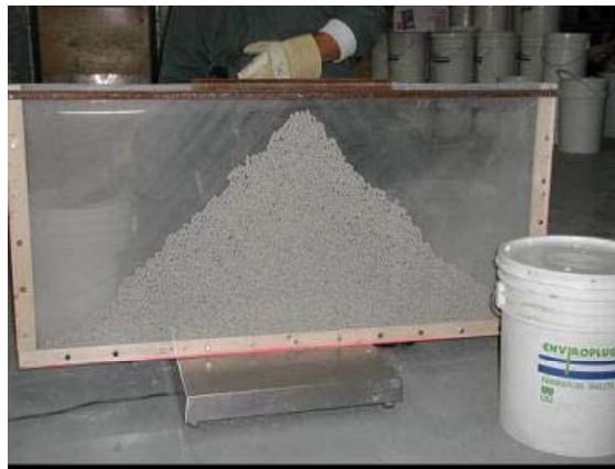
Figure 7: Placement Trial in Simulated Annular Gap [14]
