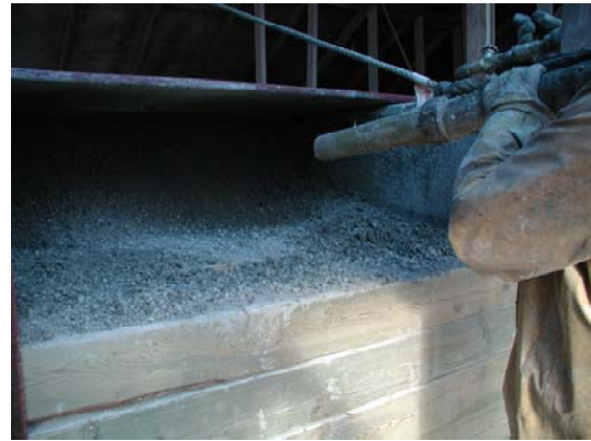
Figure 10: Light Backfill Pneumatic Emplacement Trials at AECL's URL
