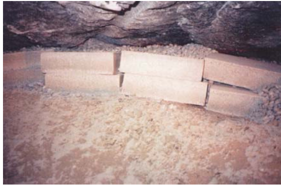
Figure 9: Filling the Crown Regions of the Backfill and Plug Test at Äspö [15]
