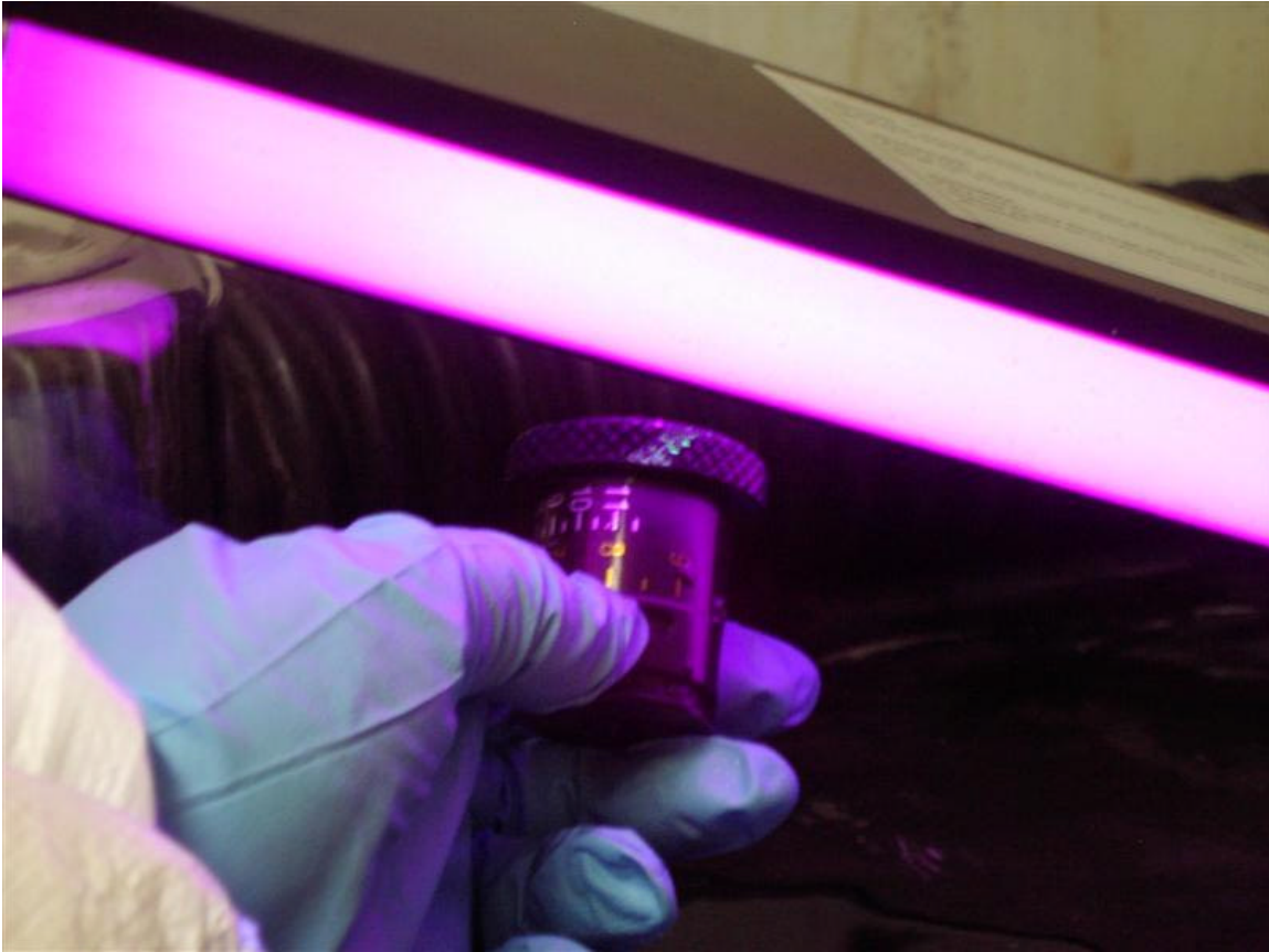
Figure 4: Sight Knob Inspection Using a Black Light
