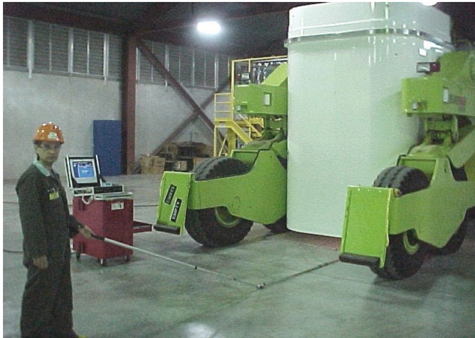
Figure 3 Remote Visual Inspection of DSC Base Plate (- digital camera being guided underneath the base plate)
