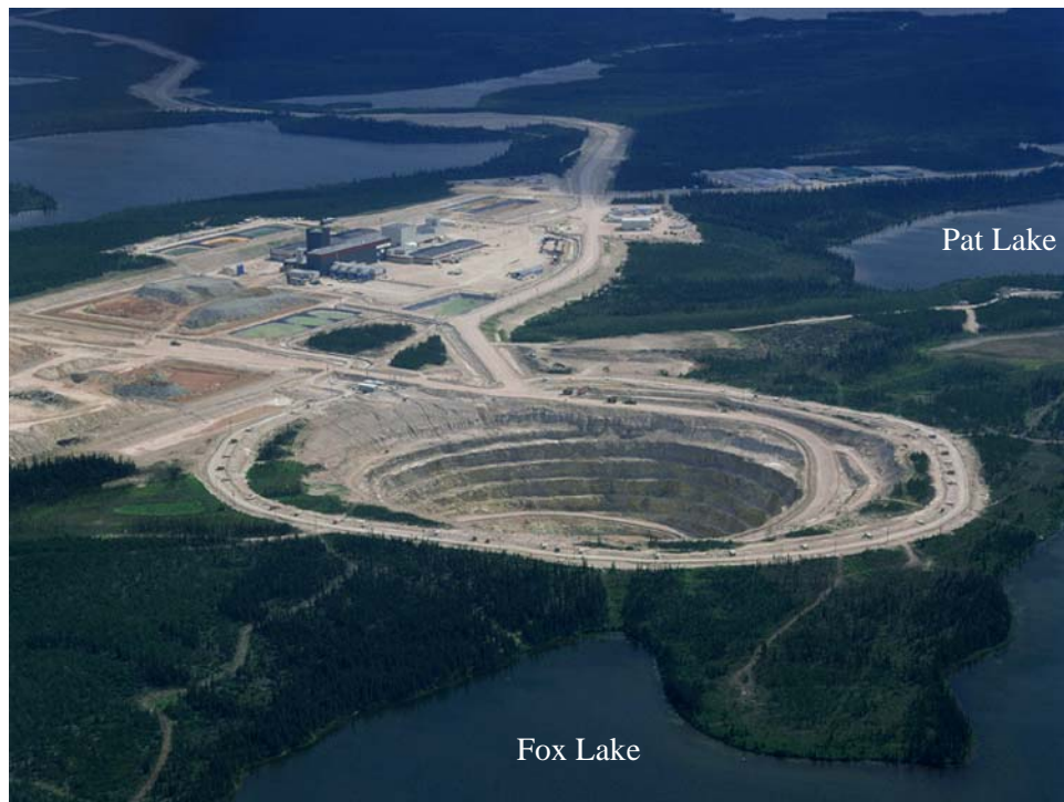
Figure 2. Aerial photograph of the McClean Lake milling site showing Fox Lake in the foreground followed by the TMF and the ore processing plant.
