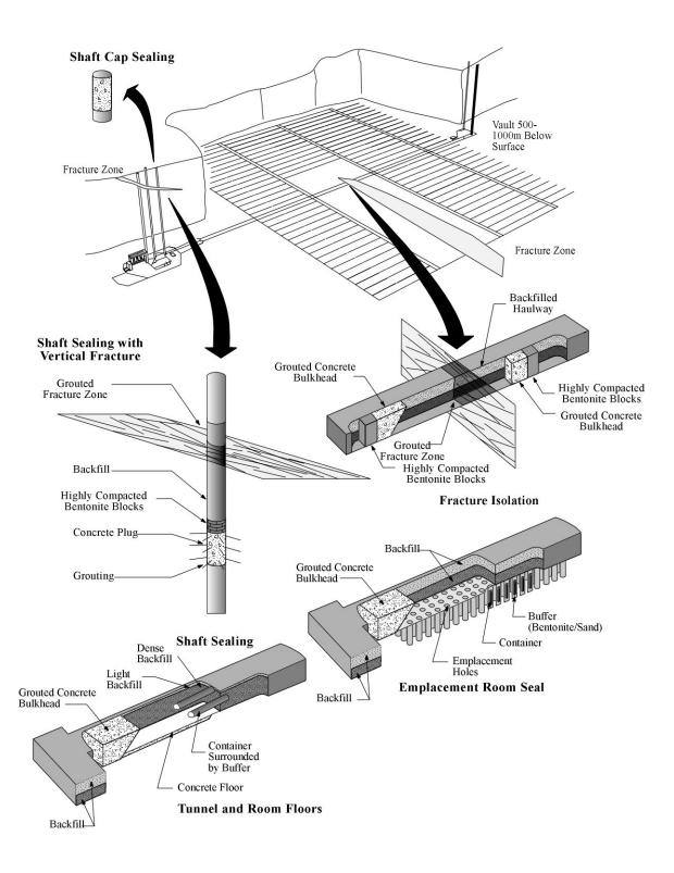
Figure 1: Potential uses of concrete in a deep geologic repository.
