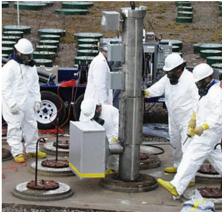
Figure 3. Hydraulic lifting apparatus installed on tile hole.
