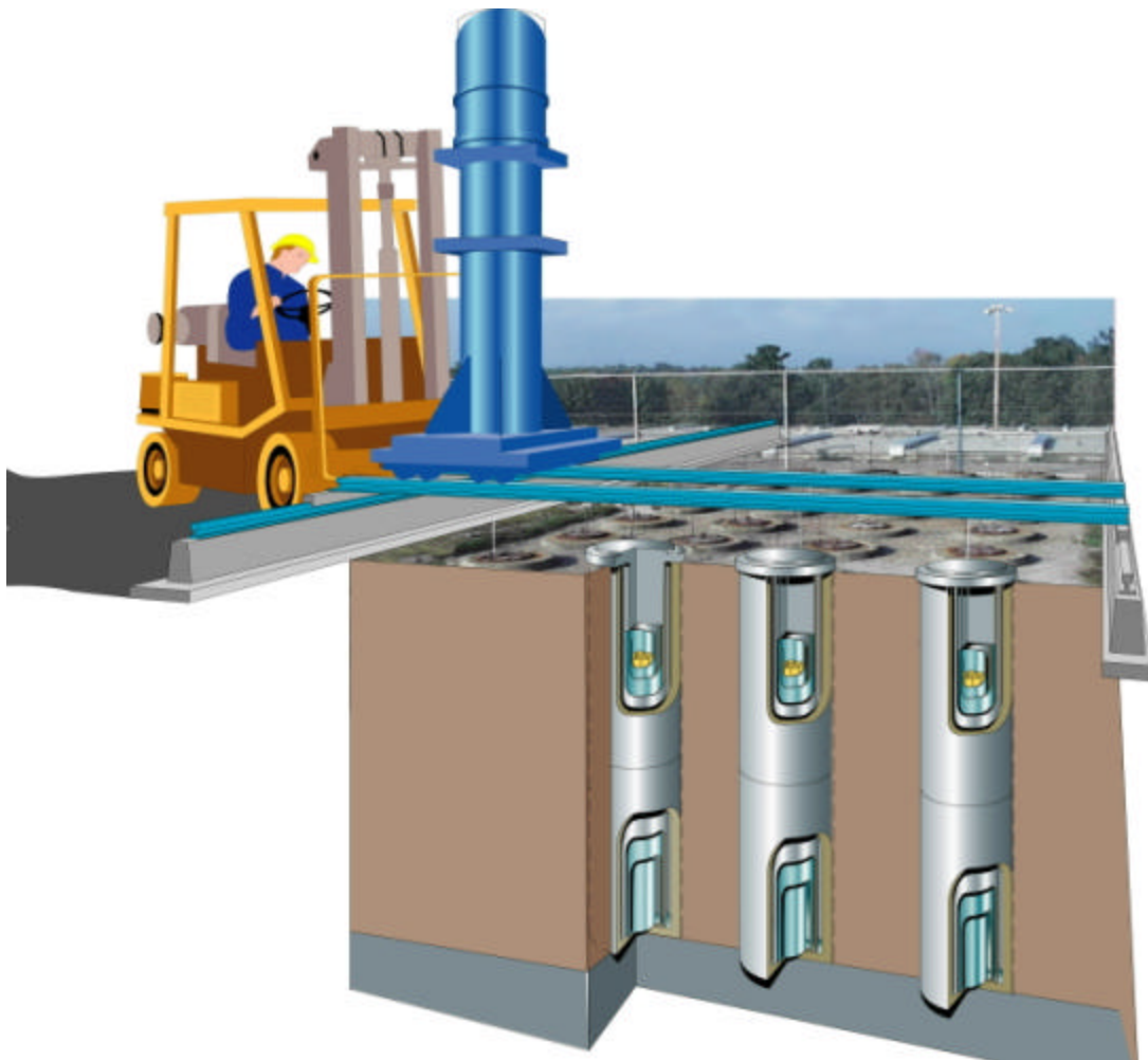
Figure 5. Concept view of the Array Bridge and FPS Retrieval Flask positioned above the tile holes array.
