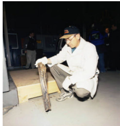
Figure 10: An empty 45-gallon drum is compacted to a 'pancake' by the high force compactor during a test.
