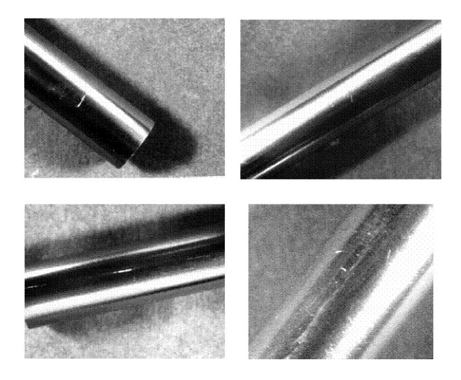
Addition of a 0.3 mm  $Ø \times 0.2$  mm deep flat bottom hole in conventional reference standards helps in identifying fine pitting on the surface of the tube for better corrosion resistance of material.
