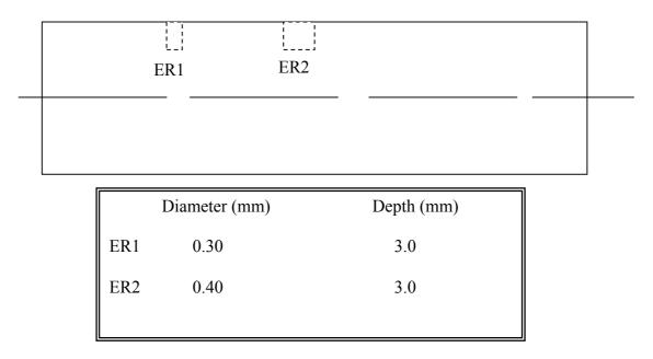
EDDY CURRENT TEST STANDARD FOR PHWR BAR
