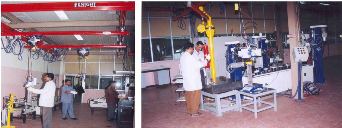
Fig.4: Air balancer type fuel bundle handling system
