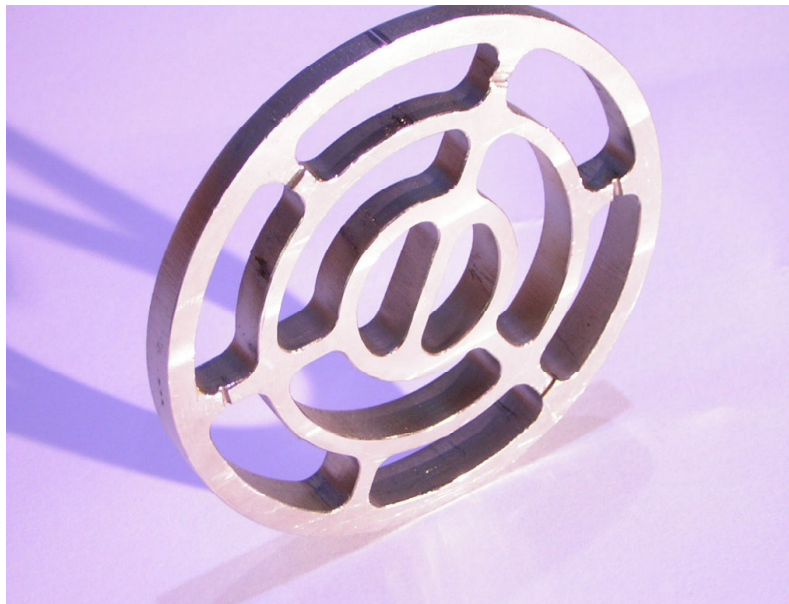
FIGURE 3 WEDGE_SHAPED END PLATE AFFIXED TO THE UPSTREAM END OF TB#2 TO SIMULATE AGED PT CONDITION
