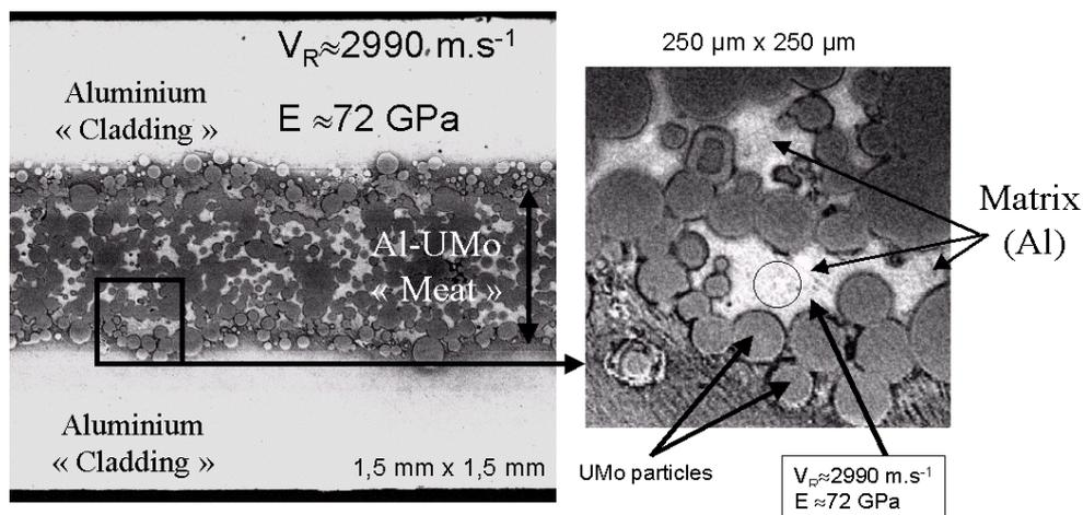
FIGURE 5 – HIGH FREQUENCY 600 MHZ ACOUSTIC PICTURE OF UMo COMPOSITE
