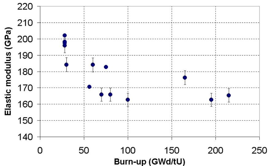
FIGURE 1 – ELASTIC MODULUS MEASURED VERSUS SIMULATED BURN-UP
