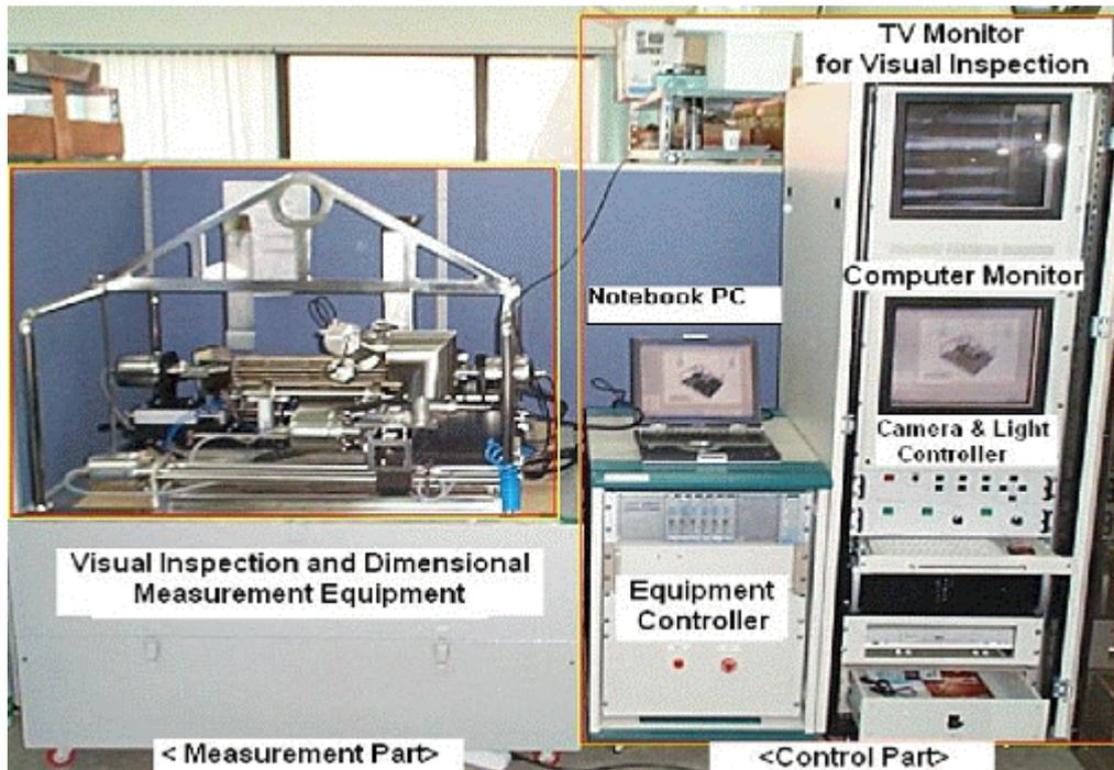
Figure 2. Overall Assembly of the In-Bay Inspection Equipment
