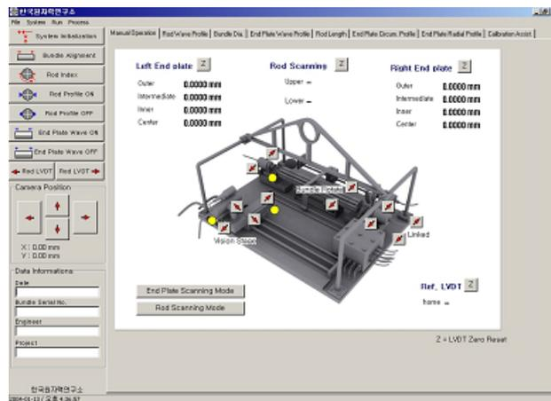
Figure 3. Main Screen of Executive Program for the In-Bay Inspection System
