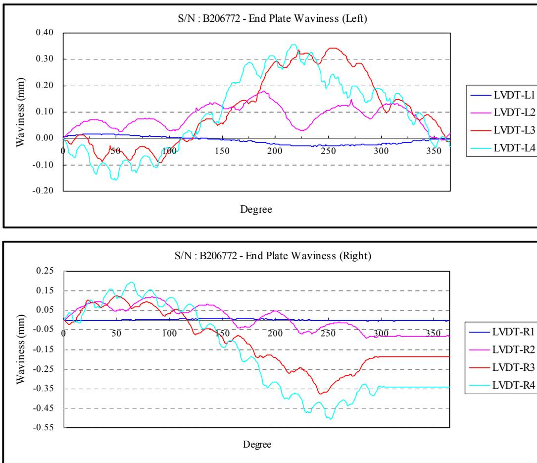
Figure 13. An Endplate Waviness Profile of the B206772 Bundle Discharge Normally from the O07 Channel of WPGS-3
