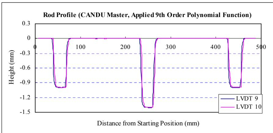
Figure 9. Axial Profile of CANDU 37-Element Fuel Master with the Calibration of the LVDT Axial Moving Structural-System
