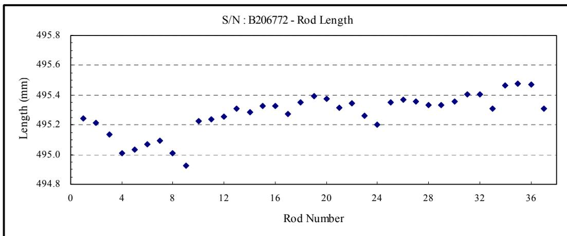
Figure 14. Element lengths over the Endplates of the B206772 Bundle Discharge Normally from the O07 Channel of WPGS-3
