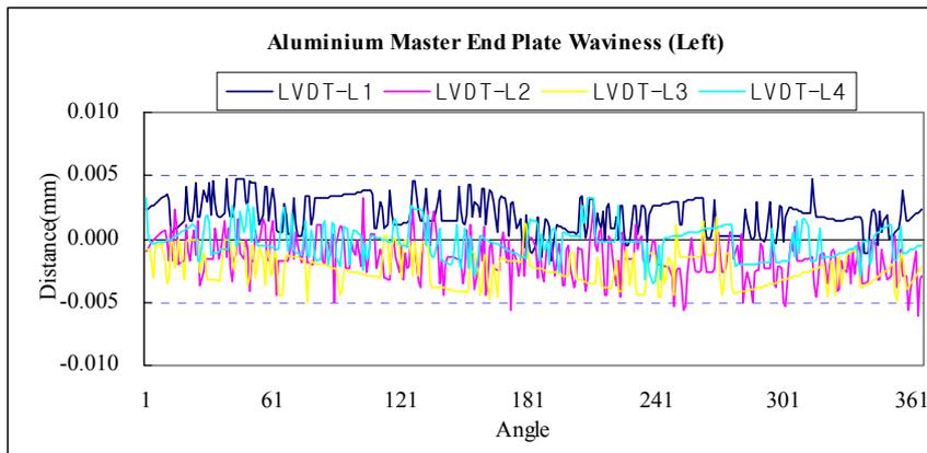
Figure 7. Waviness Profile of Left End Plane of Aluminium Master with the Calibration of the LVDT Rotational Structural-System
