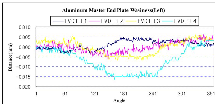
Figure 6. Waviness Profile of Left End Plane of Aluminium Master without the Calibration of the Rotational Structural-System
