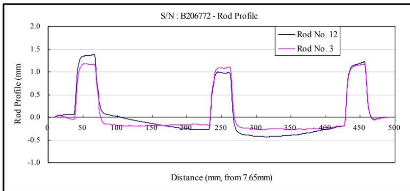
Figure 11. Axial Profile of Outer Element Bowings of the B206772 Bundle Discharge Normally from the O07 Channel of WPGS-3
