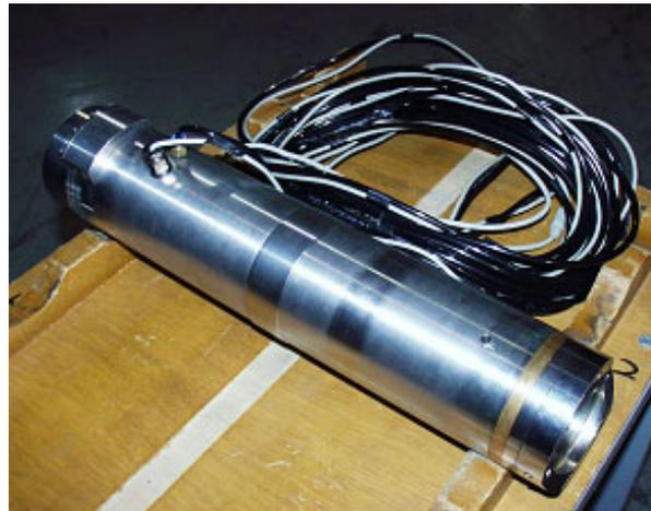
Figure 4. Standard Drum Bundle having One Step Motor and One Linear Actuator for the Calibration of LVDTs
