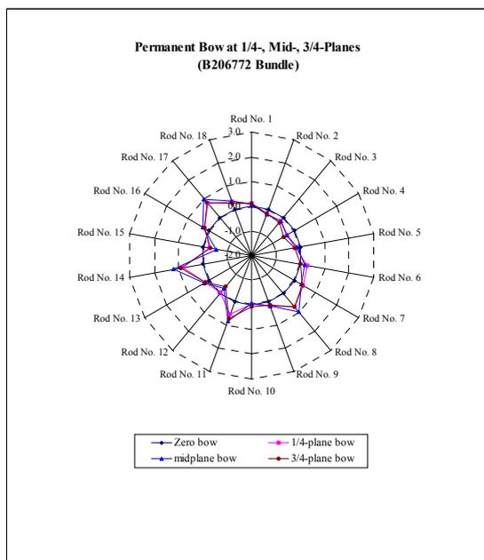
Figure 12. Radial Bundle-Profile of Outer Element Bowings of the B206772 Bundle Discharged Normally from the O07 Channel of WPGS-3
