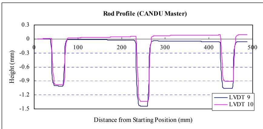
Figure 8. Axial Profile of CANDU 37-Element Fuel Master without the Calibration of the LVDT Axial Moving Structural-System
