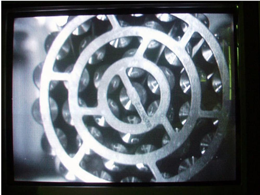
Figure 10. An Endplate Shape of the B206772 Bundle Discharged Normally from the O07 Channel of WPGS-3
