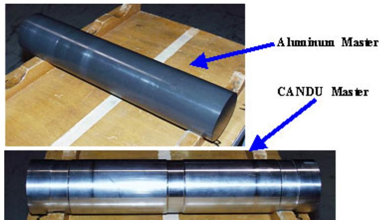
Figure 5. Aluminium Master and CANDU 37-Element Fuel Master
