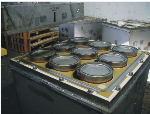
C) Global Nuclear Fuels New Powder Container (NPC)
