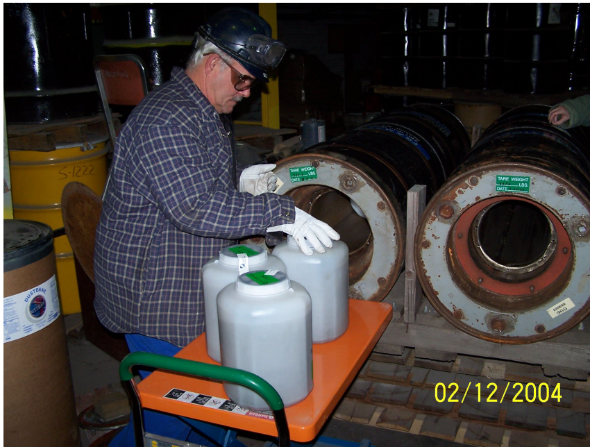
Figure 3. Loading the bottles with SEU powder into ANF250 shipping container
