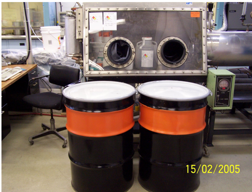
Figure 4. Overpacks for shipping BDU powder for DI
