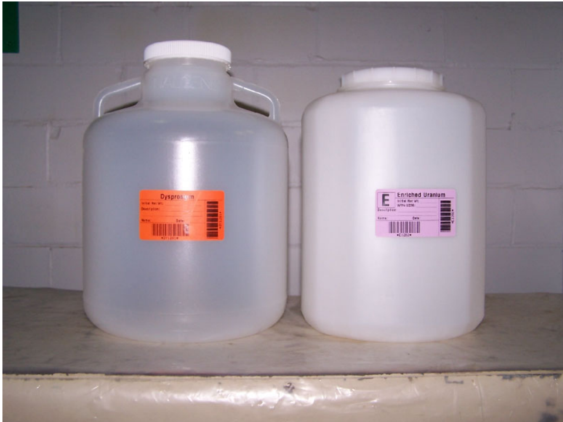
Figure 5. Different shape plastic containers for BDU (left) and SEU (right) powders
