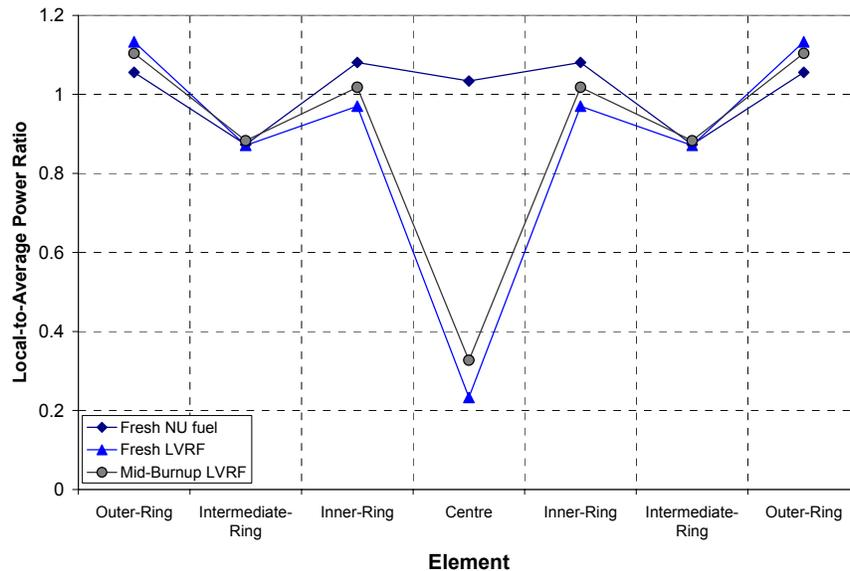
**FIGURE 4: RADIAL POWER PROFILES COVERED IN LVRF CHF TEST.**
