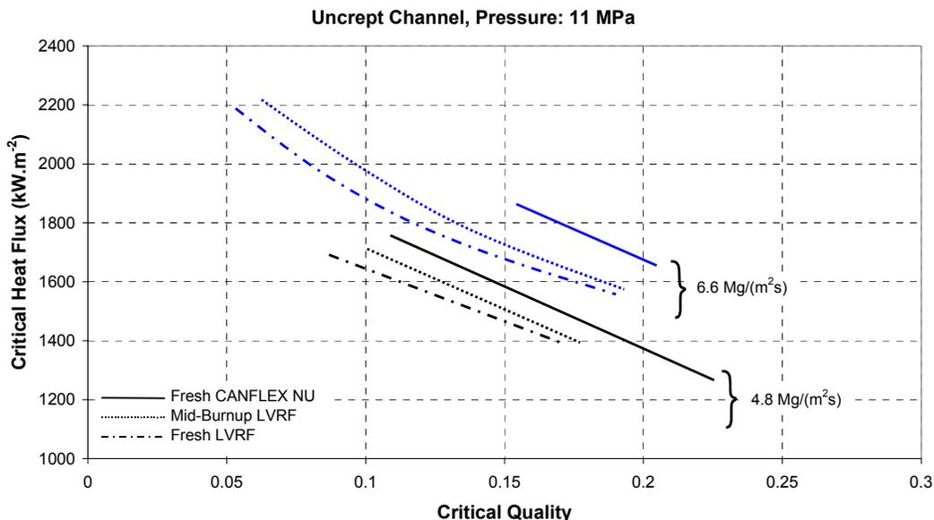
**FIGURE 6: COMPARISON OF CHF VALUES FOR VARIOUS PROFILES IN UNCREPT-CHANNEL TEST.**
