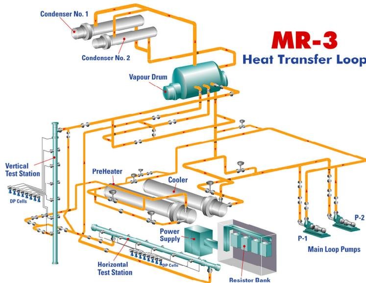
**FIGURE 2: MR-3 FREON HEAT-TRANSFER LOOP AT CRL.**
