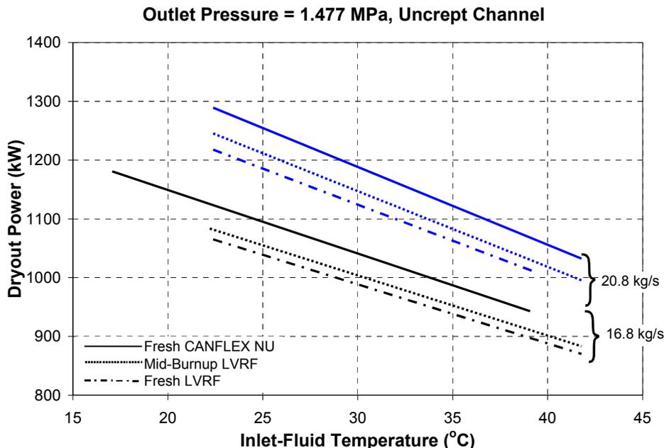
**FIGURE 5: COMPARISON OF DRYOUT POWER DATA FOR VARIOUS PROFILES.**
