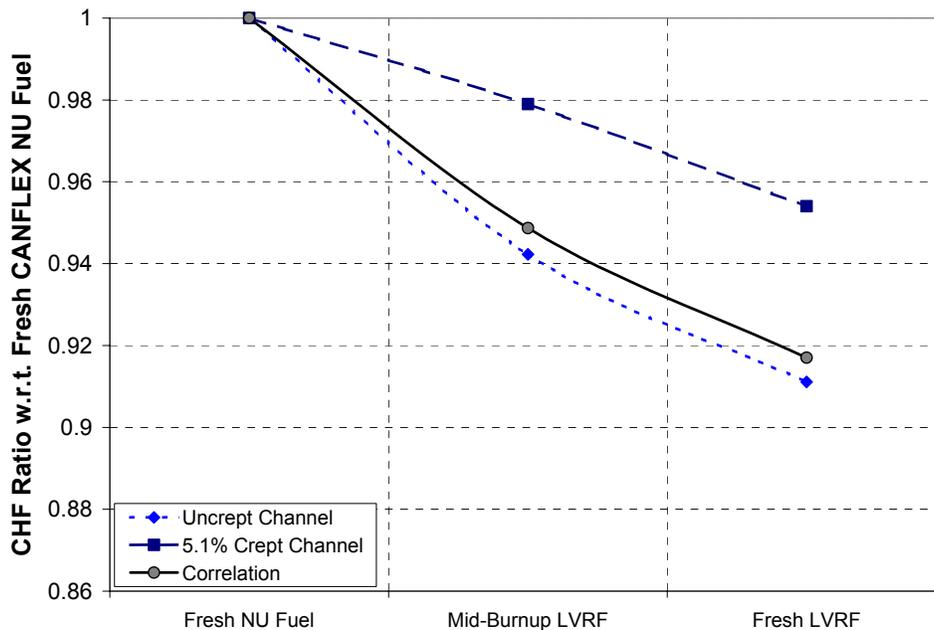
**FIGURE 7: COMPARISON OF EXPERIMENTAL CHF RATIOS FOR VARIOUS RADIAL POWER PROFILES OF LVRF BUNDLE.**
