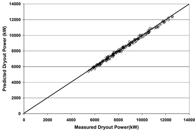
**Figure 3: Comparison of Predicted and Measured Dryout Power**
