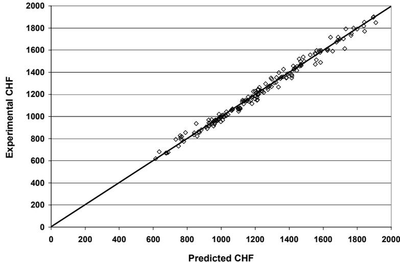
**Figure 2: Comparison of Predicted and Measured CHF Data**
