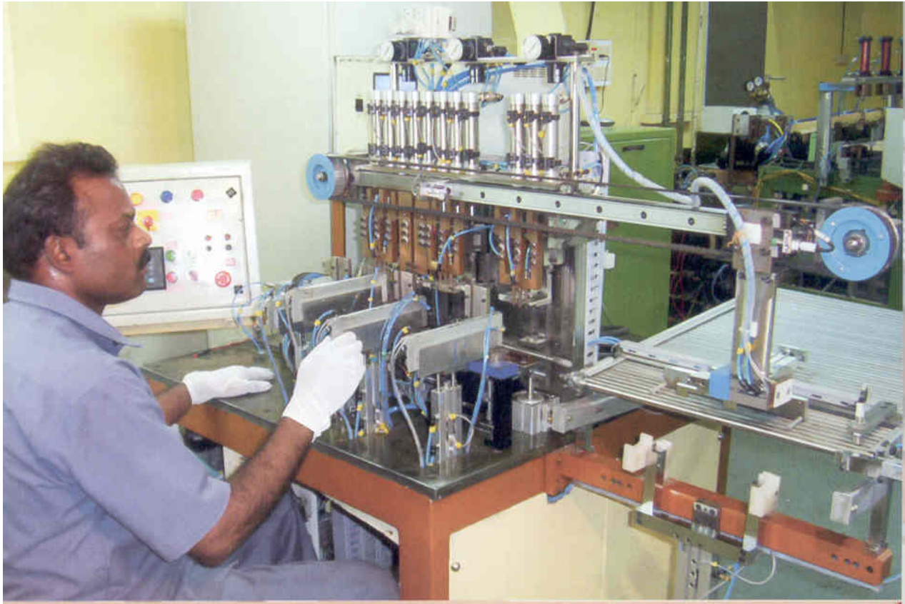
FIG 3: INTEGRATED SPACER AND BEARING PAD WELDING MACHINE
