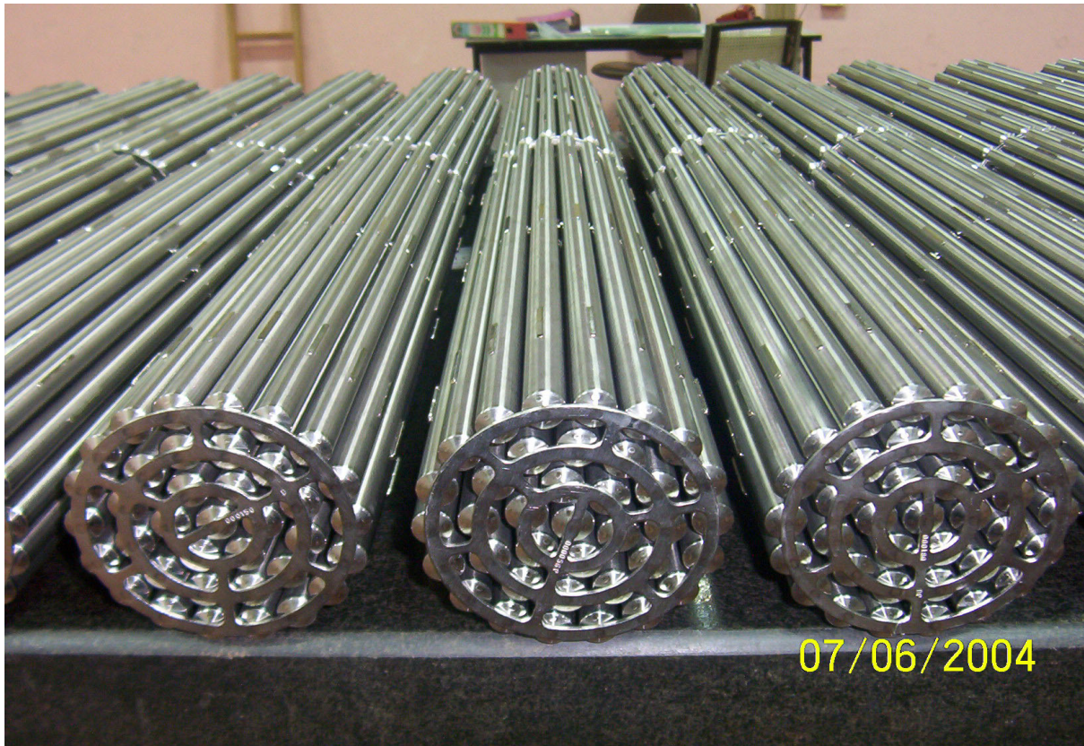
FIG 2: 37-ELEMENT FUEL BUNDLES FOR 540 MWe PHWRs
