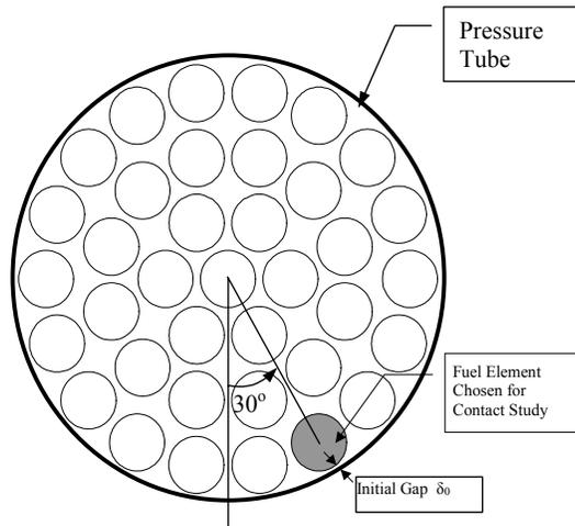
FIGURE 6 FUEL ELEMENT (SHADED) IN A FUEL BUNDLE CHOSEN FOR CONTACT STUDY
