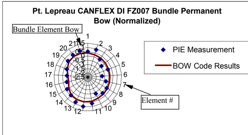
FIGURE 13 BUNDLE-ELEMENT BOW PROFILE AT MID-PLANE (WITH AVERAGE AS-FABRICATED BOW)
