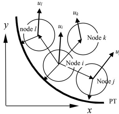
FIGURE 3 CONTACT DIRECTIONS FOR A NODE
