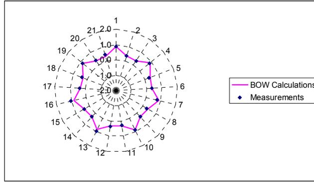
FIGURE 11 COMPARISON BETWEEN BOW CALCULATION AND DROOP MEASUREMENTS (OVERHANG SUPPORT, NORMALIZED)
