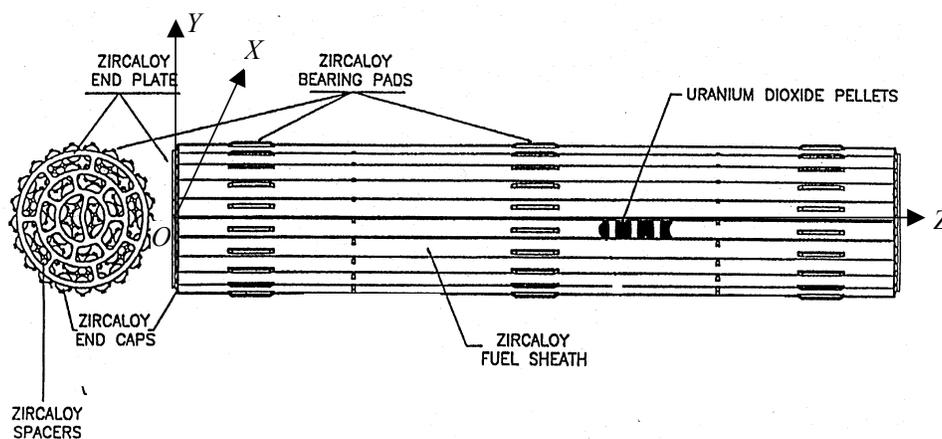
FIGURE 1 A CANFLEX 43-ELEMENT BUNDLE AND ITS GLOBAL COORDINATE SYSTEM
