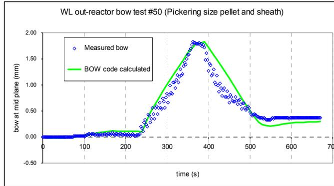
FIGURE 12 DEFLECTION OF FUEL-ELEMENT SIMULATOR AT THE MIDPLANE: WL TEST #50
