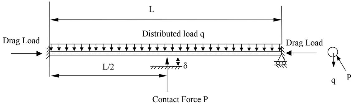
FIGURE 7 A CLAMPED BEAM SUBJECTED TO CONTACT CONSTRAINT AT MIDPOINT
