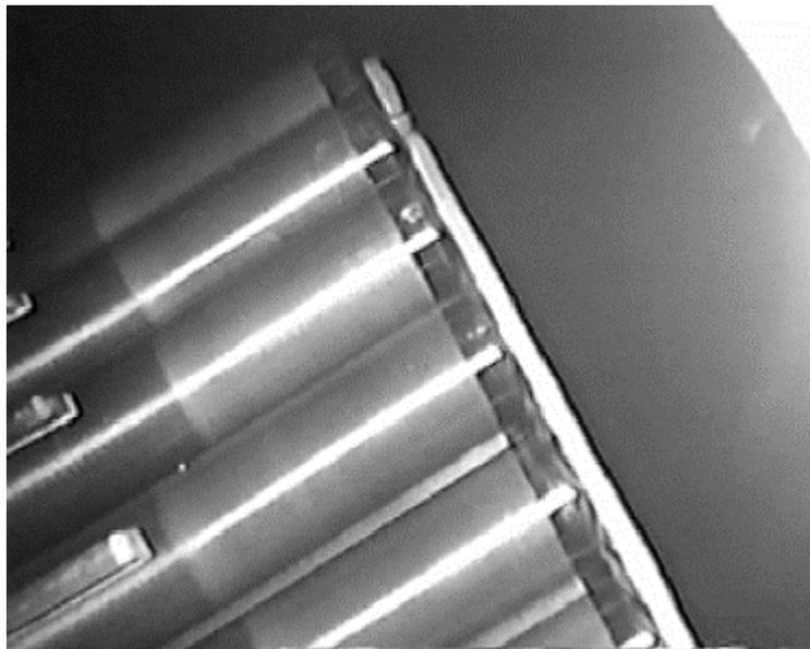
**Figure 8. CANFLEX-NU KF0119 Bundle - Endcaps-Endplate Welding**
