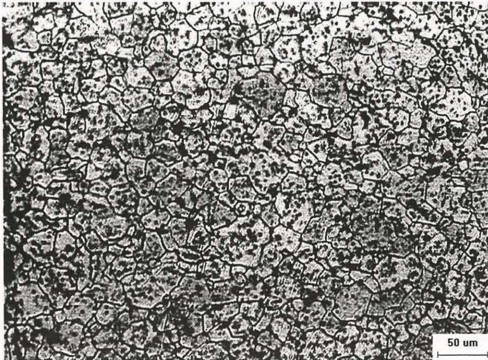
FIGURE 3. MICROSTRUCTURE OF SINTERED DUPIC PELLET
