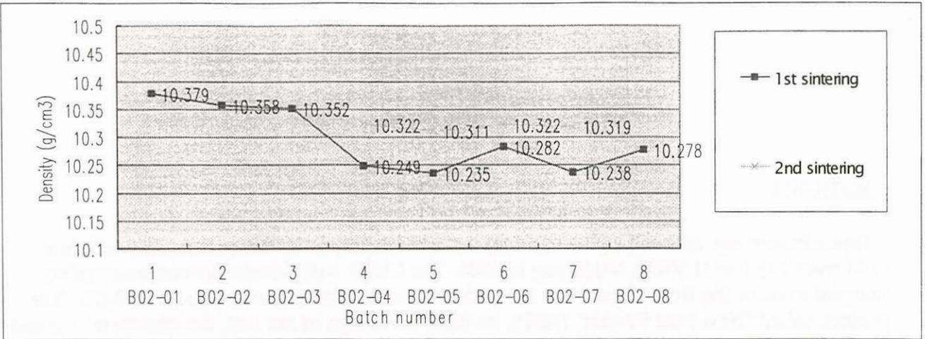
FIGURE 2. DENSITY OF SINTERED DUPIC PELLETS
