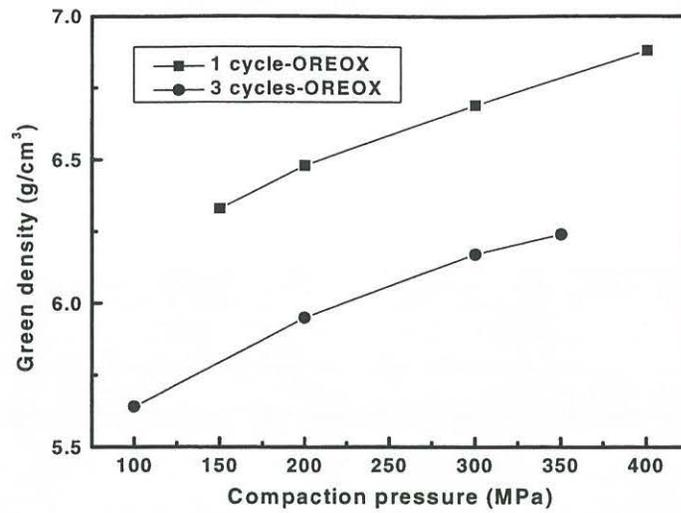
FIGURE 2. THE VARIATION OF GREEN DENSITIES WITH COMPACTING PRESSURE
