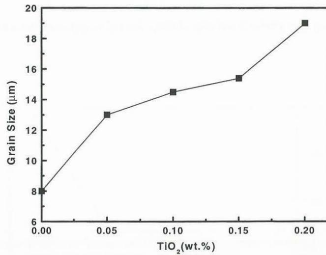
FIGURE 7. THE VARIATION OF GRAIN SIZE WITH TiO<sub>2</sub> CONCENTRATION
