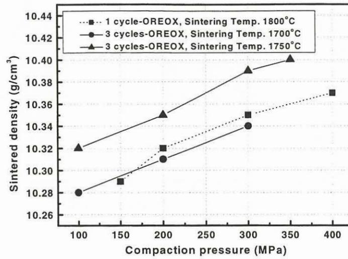
FIGURE 4. EFFECTS OF THE COMPACTING PRESSURE ON SINTERED DENSITIES
