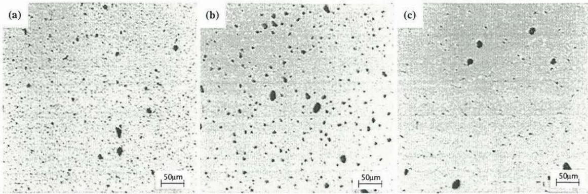
FIGURE 6. MICROSTRUCTURES OF SINTERED PELLETS WITH TiO<sub>2</sub> ADDITIONS; (a) 0 wt.%, (b) 0.15 wt.%, (c) 0.2 wt.%
