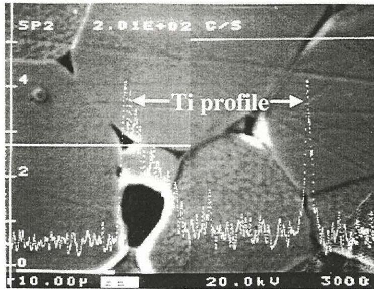
FIGURE 8. SEM MICROGRAPH SHOWING THE SECONDARY PHASE FORMED ON THE GRAIN BOUNDARY
