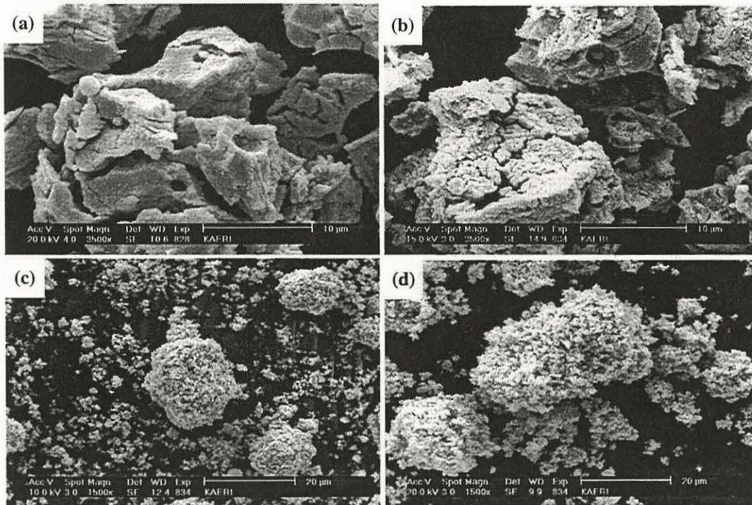
FIGURE 1. MORPHOLOGIES OF POWDERS; (a) 1 CYCLE-OREOX POWDER, (b) 3 CYCLES- OREOX POWDER, (c) 120 MINUTES MILLING, 1 CYCLE-OREOX POWDER, (d) 15 MINUTES MILLING, 3 CYCLES-OREOX POWDER
