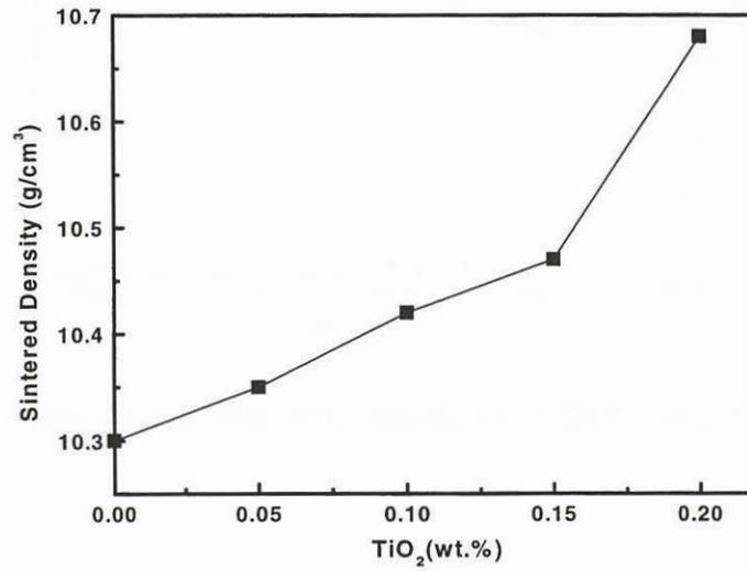
FIGURE 5. THE VARIATION OF SINTERED DENSITY WITH TiO<sub>2</sub> CONCENTRATION
