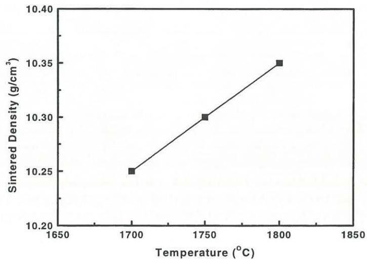
FIGURE 3. THE VARIATION OF SINTERED DENSITY OF THE 1 CYCLE-OREOX POWDER WITH SINTERING TEMPERATURE (COMPACTING PRESSURE: 300 MPa)
