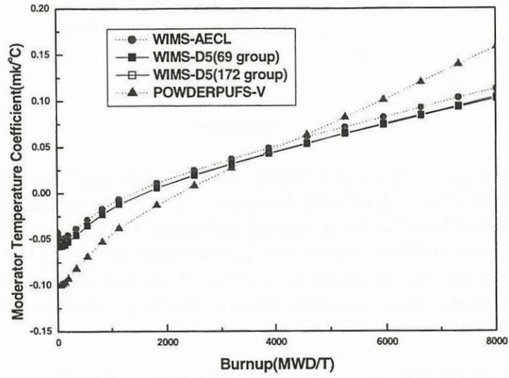
Figure 6 Moderator temperature coefficient
