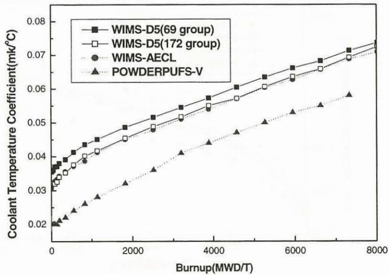
Figure 3 Coolant temperature coefficient
