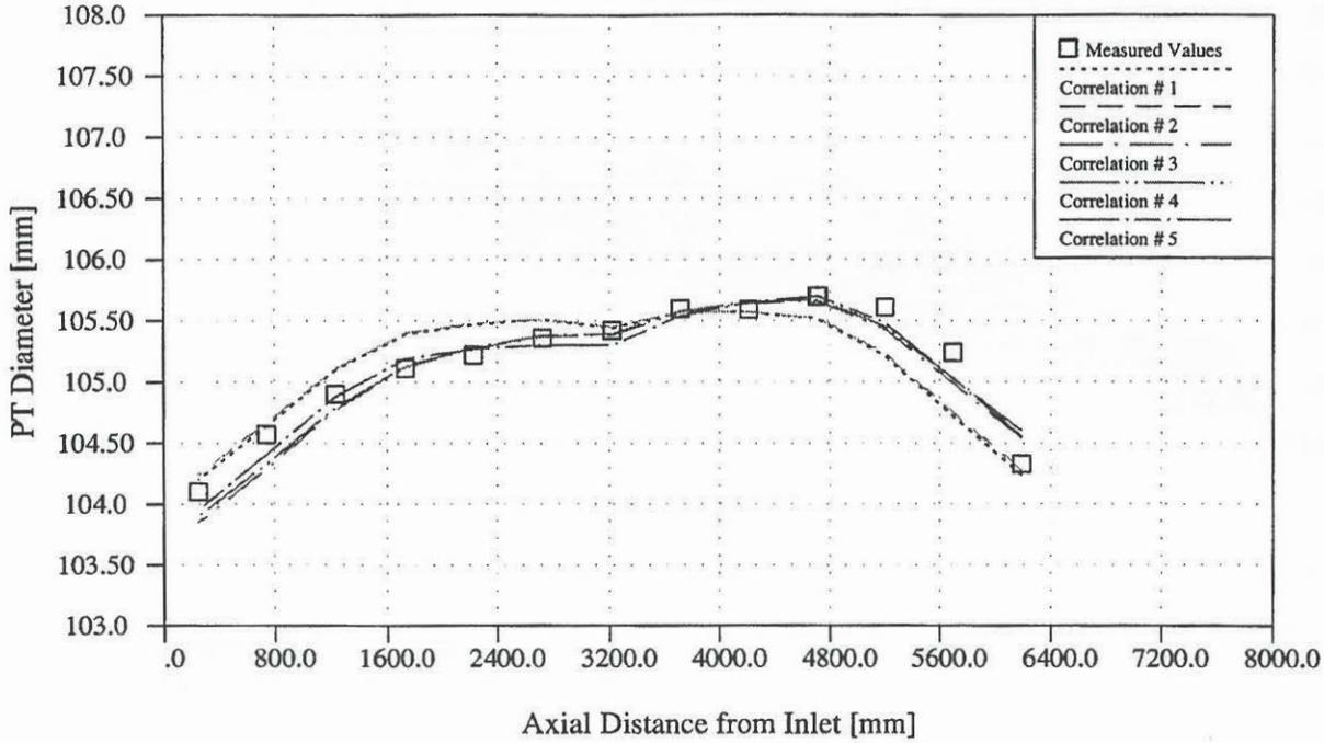
**FIGURE 4 : COMPARISON BETWEEN PREDICTED AND MEASURED PRESSURE TUBE DIAMETER PROFILES
