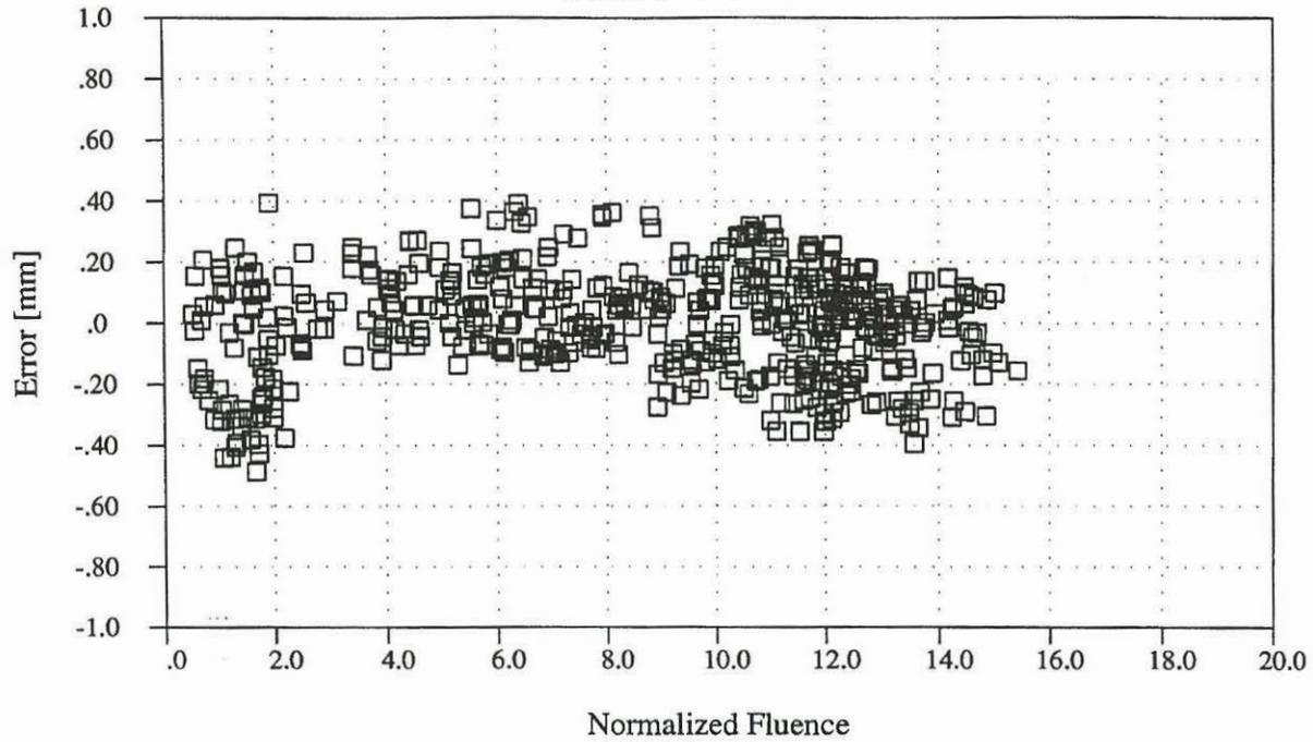
**FIGURE 10 : ERROR IN PRESSURE TUBE DIAMETER AS FUNCTION OF FLUX
