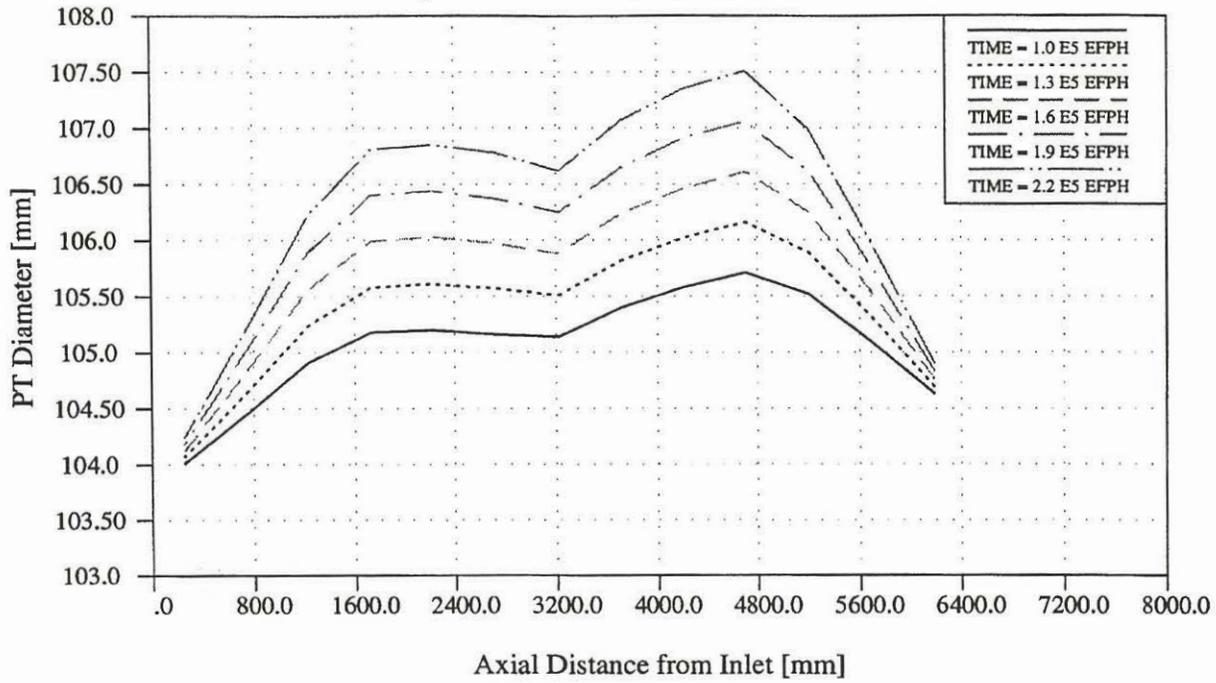
**FIGURE 18 : PREDICTED PRESSURE TUBE DIAMETRAL STRAIN PROFILES AS FUNCTION OF TIME
