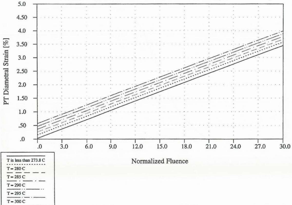
**FIGURE 17 : PREDICTED PRESSURE TUBE DIAMETER PROFILES AS FUNCTION OF TIME
