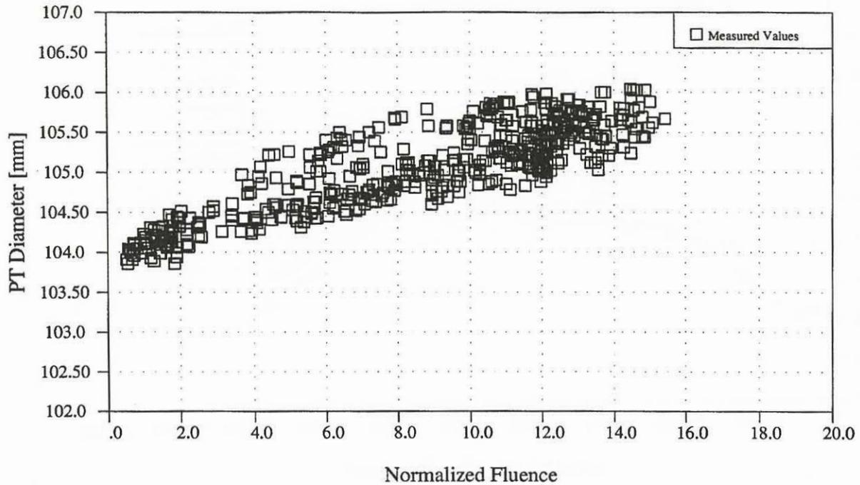
**FIGURE 2 : MEASURED PRESSURE TUBE DIAMETER AS FUNCTION OF FLUX**
