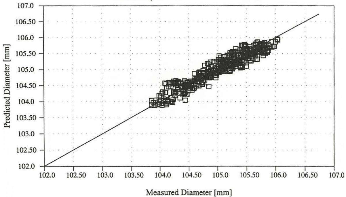
**FIGURE 7 : COMPARISON BETWEEN MEASURED AND PREDICTED MAXIMUM PRESSURE TUBE DIAMETERS
