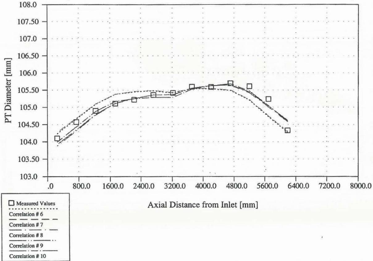
**FIGURE 5 : COMPARISON BETWEEN MEASURED AND PREDICTED PRESSURE TUBE DIAMETERS
