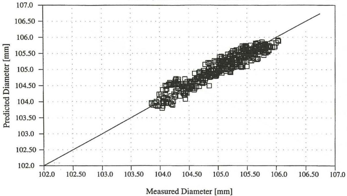
**FIGURE 6 : COMPARISON BETWEEN MEASURED AND PREDICTED PRESSURE TUBE DIAMETERS
