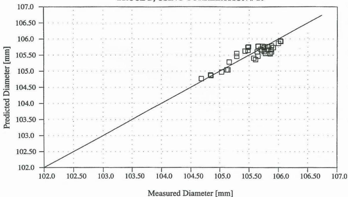
**FIGURE 8 : ERROR IN PREDICTED PRESSURE TUBE DIAMETER AS FUNCTION OF MEASURED DIAMETER
