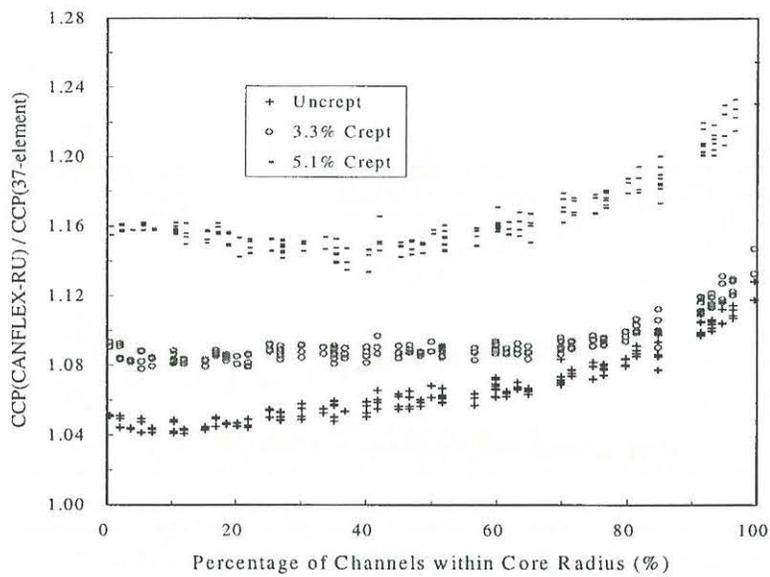
Figure 9. Comparison of the CCPs for the CANFLEX-RU Bundle Attached with the High Bearing Pads with Those for the 37-element Bundle
