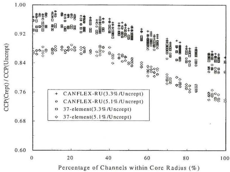
Figure 11. Comparison of the CCPs for the RU Bundle Attached with the High Bearing Pads in the 3.3% and 5.1% Crept Channels with Those in the Uncrept Channel
