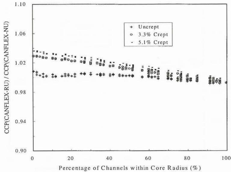
Figure 6. Comparison of the CCPs for the RU Bundle Attached with the Low Bearing Pads with Those for the NU Bundle with the Low Bearing Pads
