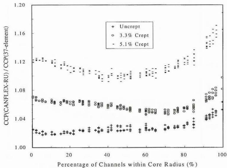
Figure 7. Comparison of the CCPs for the CANFLEX-RU Bundle Attached with the Low Bearing Pads with Those for the 37-element Bundle
