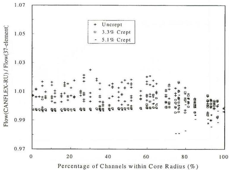
Figure 4. Comparison of Flow Rates for CANFLEX-RU Bundle with Flow Rates for the 37-element Bundle in the Uncrept, 3.3% and 5.1% Crept Channels
