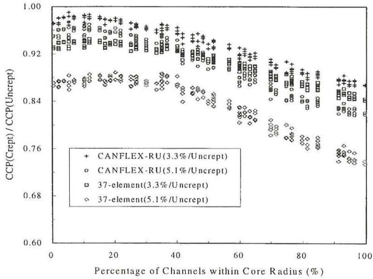
Figure 10. Comparison of the CCPs for the RU Bundle Attached with the Low Bearing Pads in the 3.3% and 5.1% Crept Channels with Those in the Uncrept Channel
