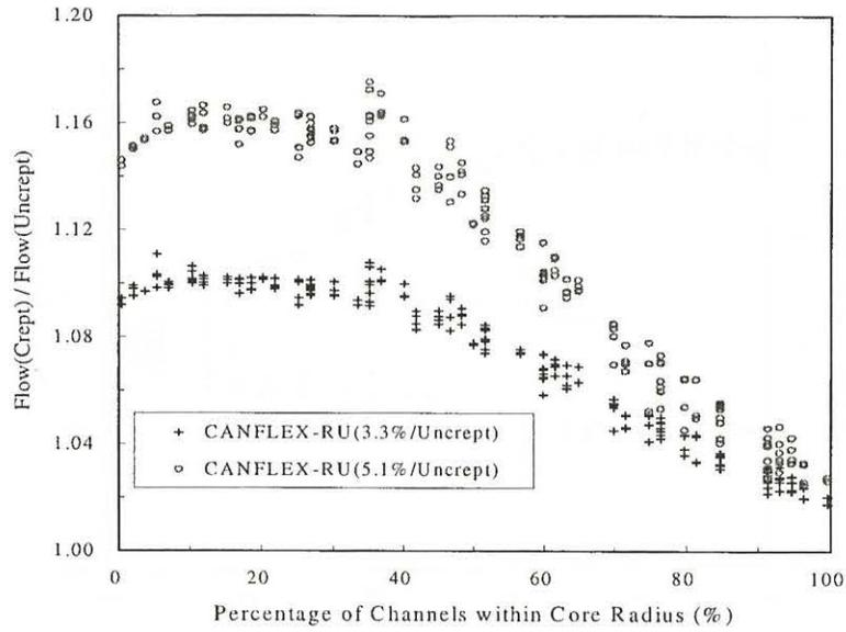
Figure 3. Comparison of Flows in the Crept Channels with Flows in the Uncrept Channel
