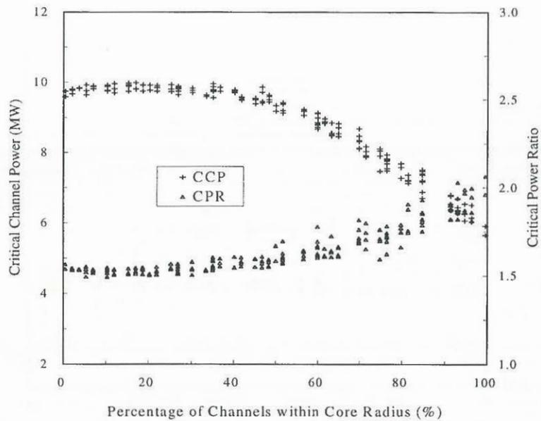
(b) In the Uncrept Channel with the CANFLEX-RU Bundle Attached with the High Bearing Pads
