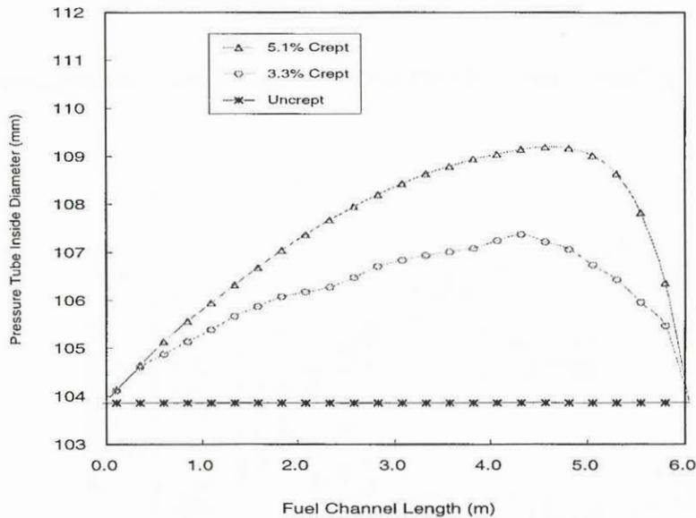
Figure 1. Axial Profiles of Pressure Tube Diametral Creep Models
