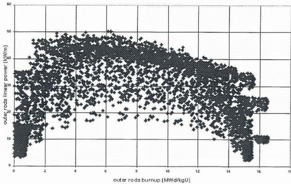
**Figure 6: Linear Powers vs Rod Burnups for a Representative Instantaneous Burnup Distribution of a Two Burnup Region SEU Core, with 4 bs Refuelling**
