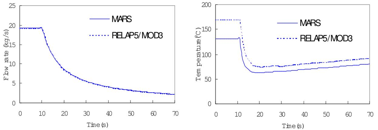
Figure 8. Comparison of flow rate and fuel temperature for RELAP5 and MARS-h
