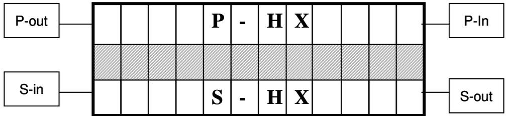
Fig. 3 Nodalization for a plate heat exchanger simulation
