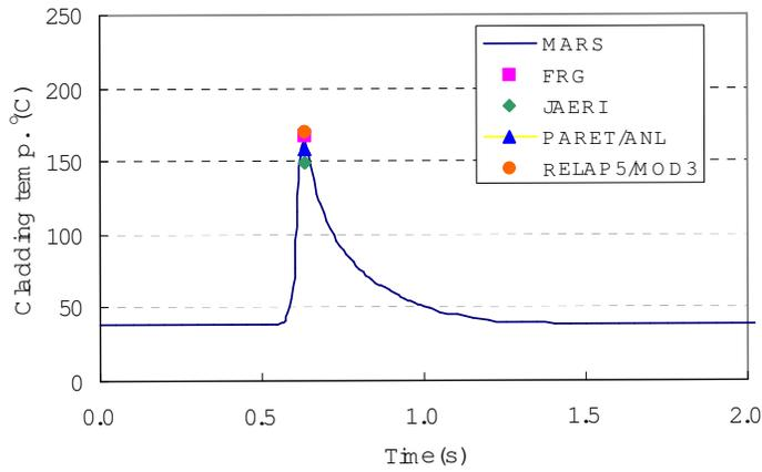
Fig. 9 Predicted peak cladding temperature at reactivity induced transient
