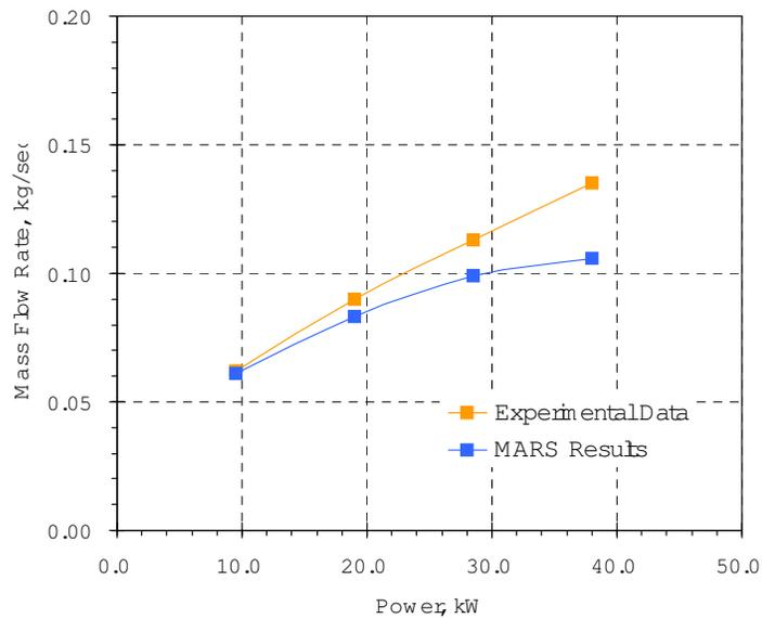
Fig. 6 Comparison of the predicted to the measured flow rate for each power level
