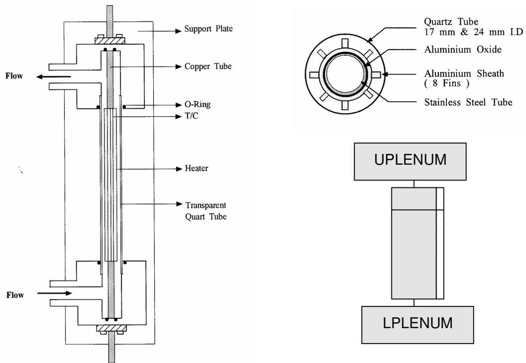
Fig. 1 Test section of single pin heat transfer experiment and nodalization for MARS-h
