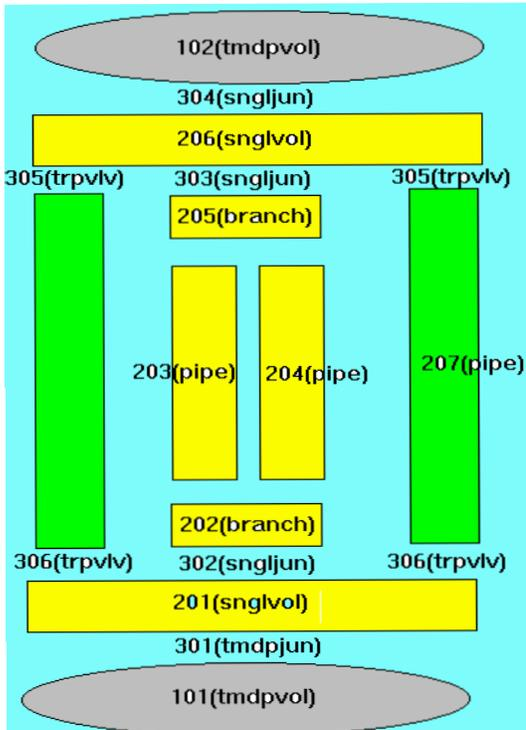
Figure 8. Nodalization of SPERT for MARS-h simulation
