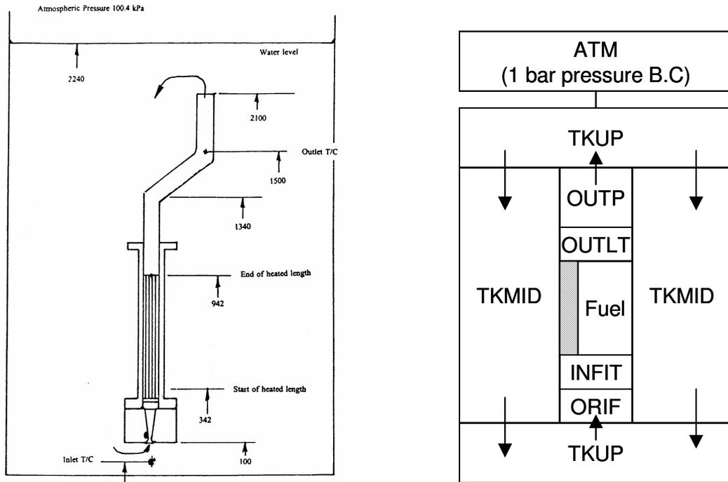
Fig. 5 Schematics of test facility and nodalization for MARS-h simulation
