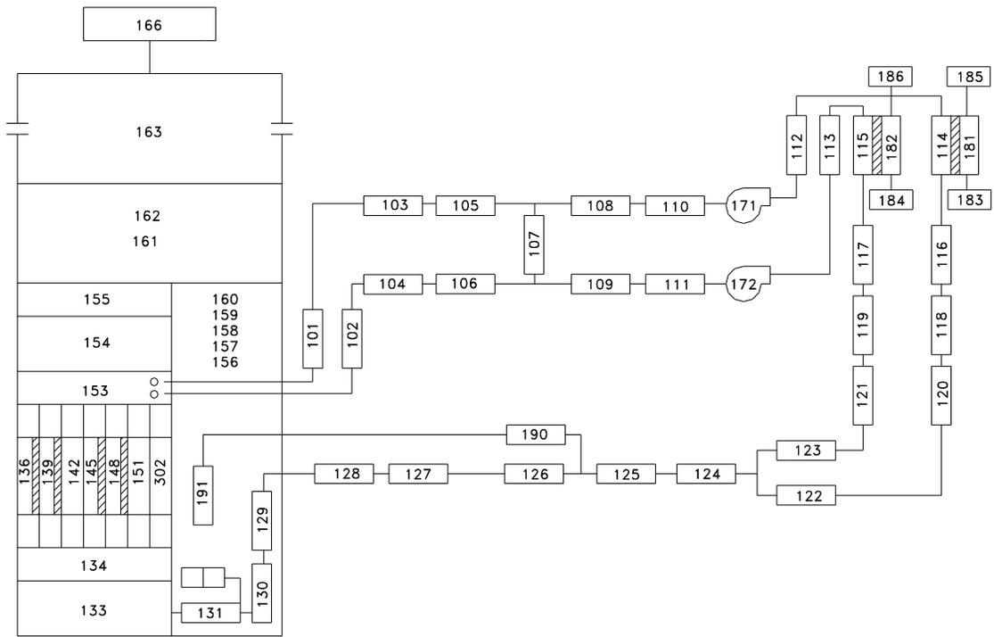
Figure 7. Nodalization of HANARO for MARS-h
