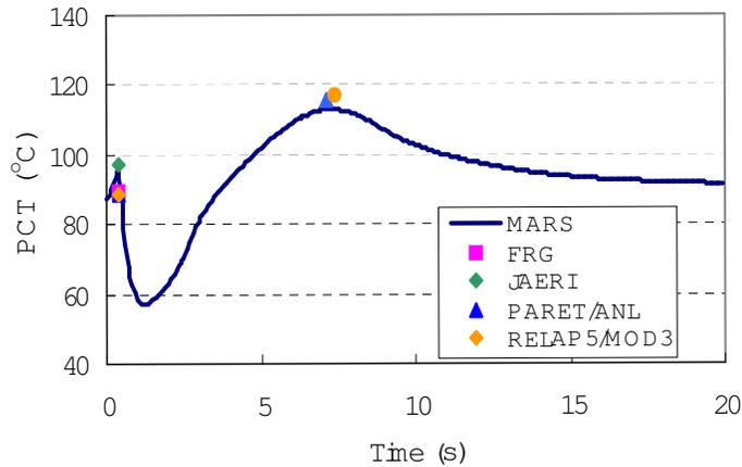
Fig. 10 Predicted peak cladding temperature at loss of flow transient
