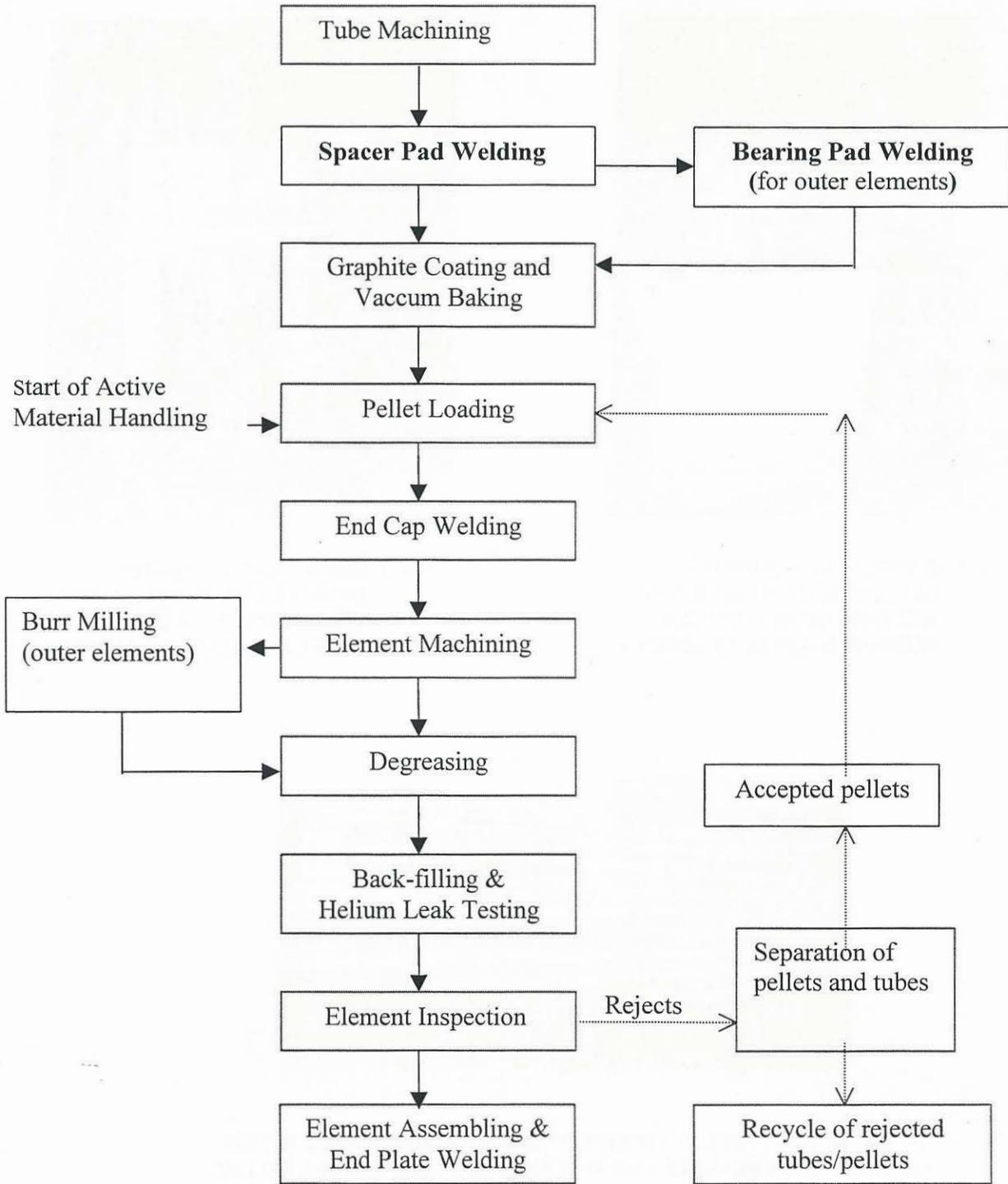
FIG 5 : NEW PROCESS FLOW SHEET FOR MANUFACTURING PHWR 220 FUEL BUNDLE
