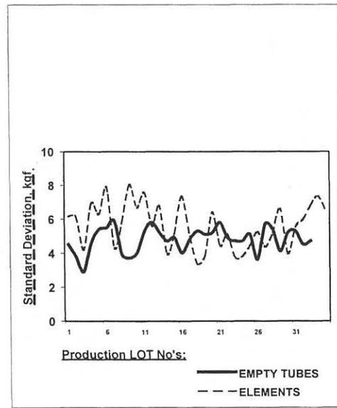
FIG 9 : COMPARISON OF STANDARD DEVIATION OF BEARING PAD WELDS
