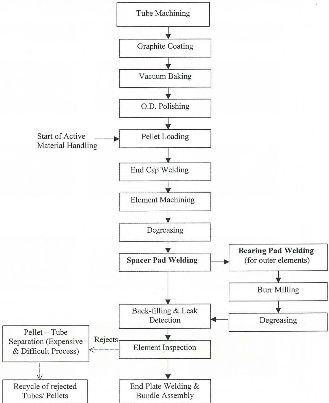
FIG 1: CONVENTIONAL PROCESS FLOW SHEET FOR MANUFACTURING 220 MWe PHWR FUEL ASSEMBLY.
