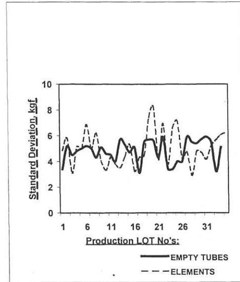
FIG 7: COMPARISON OF STANDARD DEVIATION OF S PACER PAD WELDS
