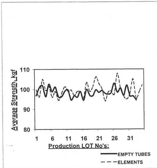
FIG 8 : COMPARISON OF AVERAGE WELD STRENGTH OF BEARING PAD WELDS
