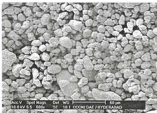
Fig.2 c. Agglomerates shape and size distribution of \text{UO}_2 produced via Spray dried ADU
