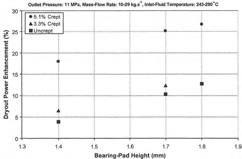
Figure 14: Dryout-power enhancement for CANFLEX bundles of various bearing-pad heights.
