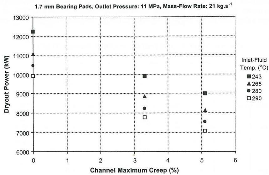
Figure 8: Effect of channel creep on dryout power.
