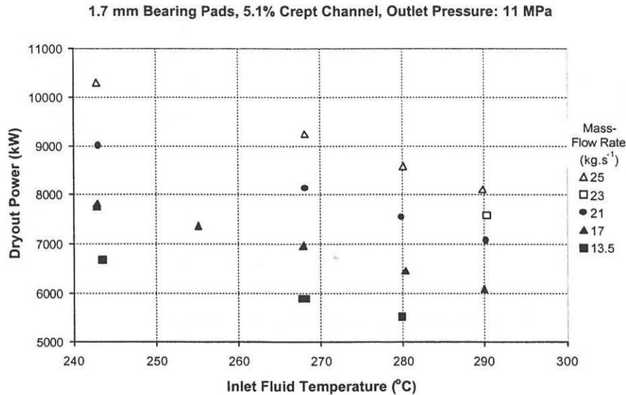
Figure 7: Dryout-power data for a CANFLEX bundle string with 1.7 mm bearing pads in the 5.1% crept channel.
