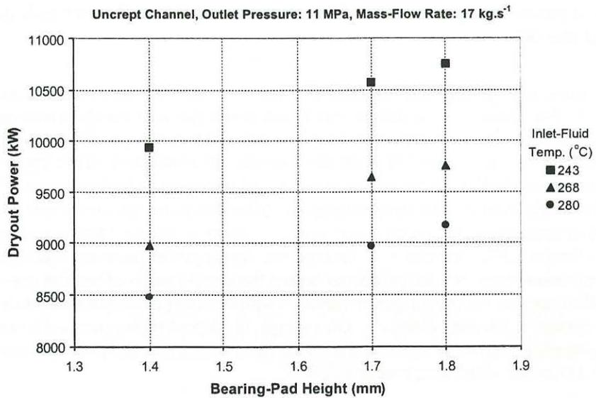
Figure 9: Effect of bearing-pad height on dryout power in the uncrept channel.
