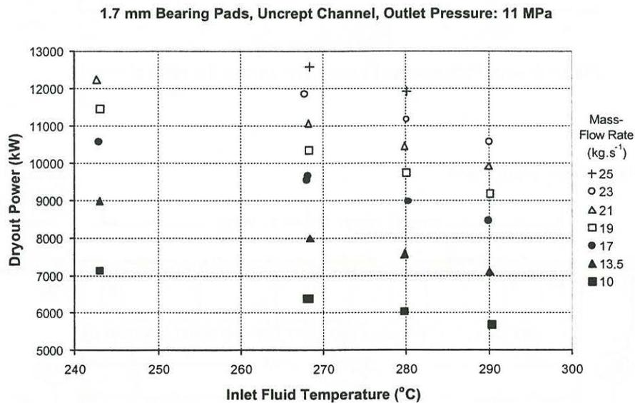
Figure 6: Dryout-power data for a CANFLEX bundle string with 1.7 mm bearing pads in the uncrept channel.
