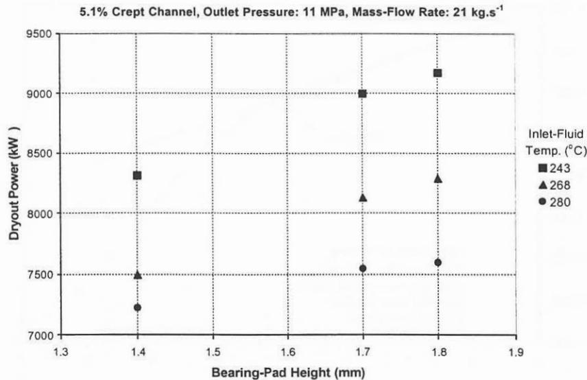
Figure 10: Effect of bearing-pad height on dryout power in the 5.1% crept channel.
