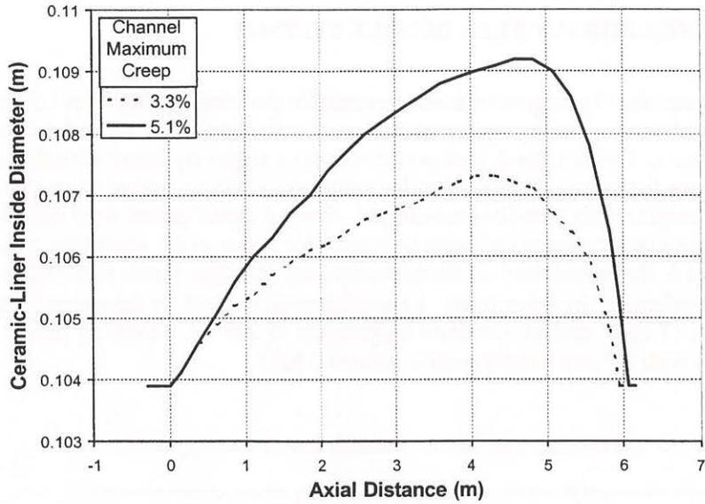
Figure 4: Axial variations of inside diameter in the crept channels.
