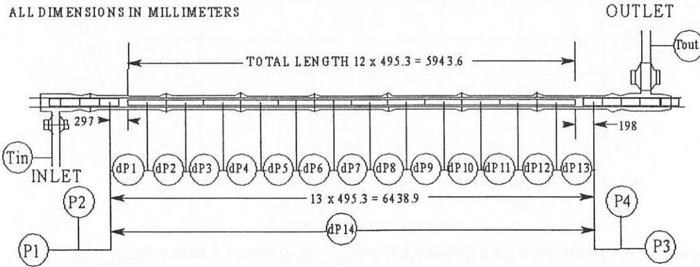
Figure 5: A schematic diagram of the test station in the high-pressure steam-water loop at Stern Laboratories.
