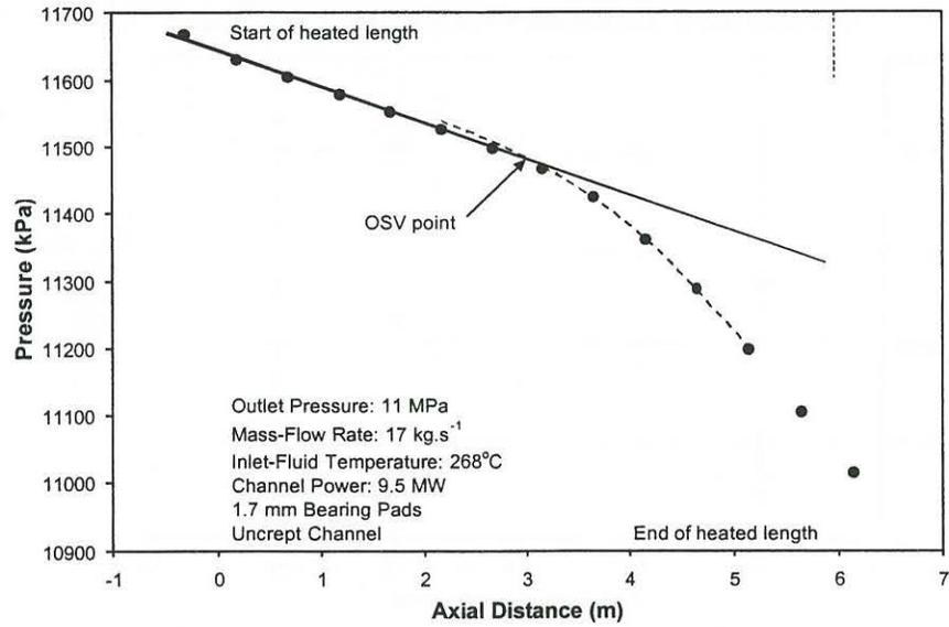
Figure 11: Pressure distribution along the channel.
