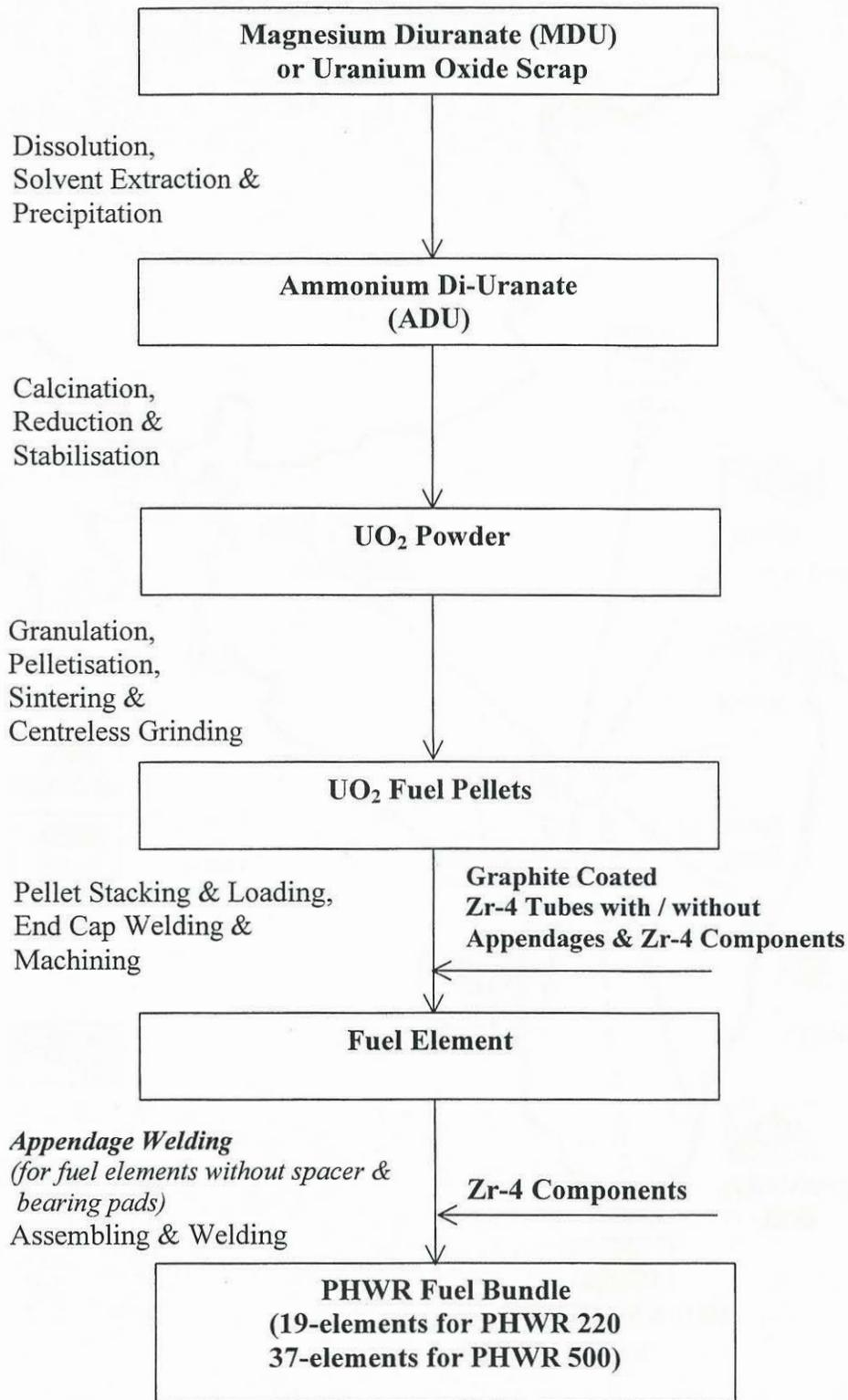
FIG 2: FLOWSHEET FOR MANUFACTURING PHWR FUEL BUNDLES AT NFC
