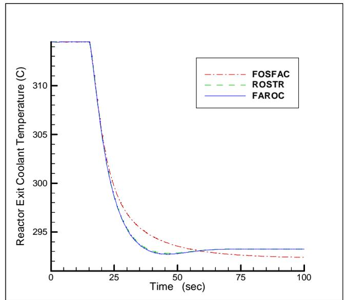
Fig. 10. Reactor exit coolant temperature for 100% to 10% power level change
