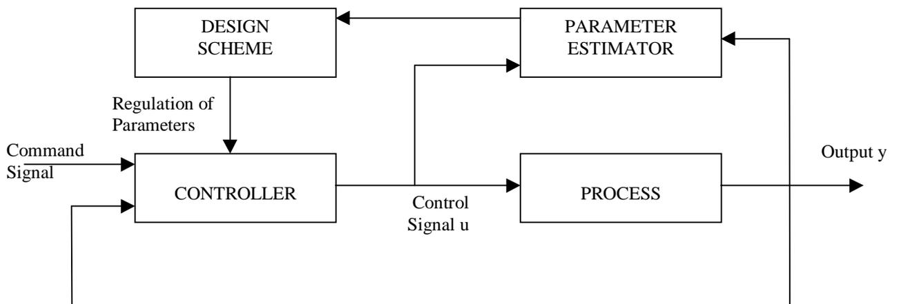
Fig. 1. Block diagram of a self-tuning regulator (STR)
