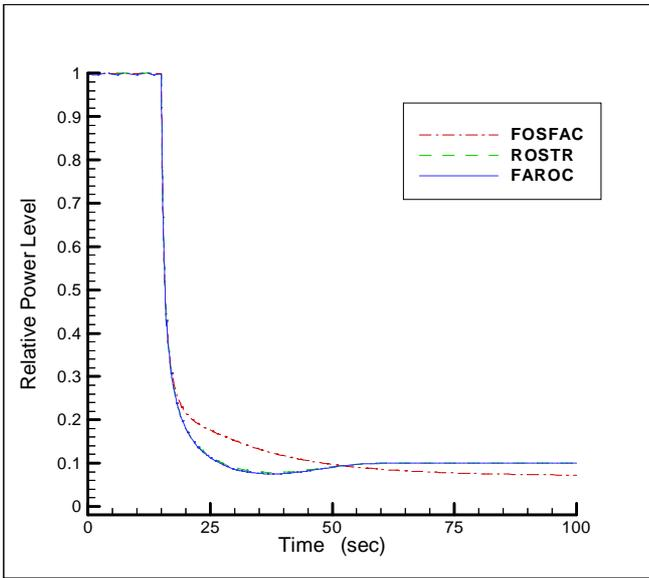
Fig. 7. Very large step change of power level from 100% to 10%.
