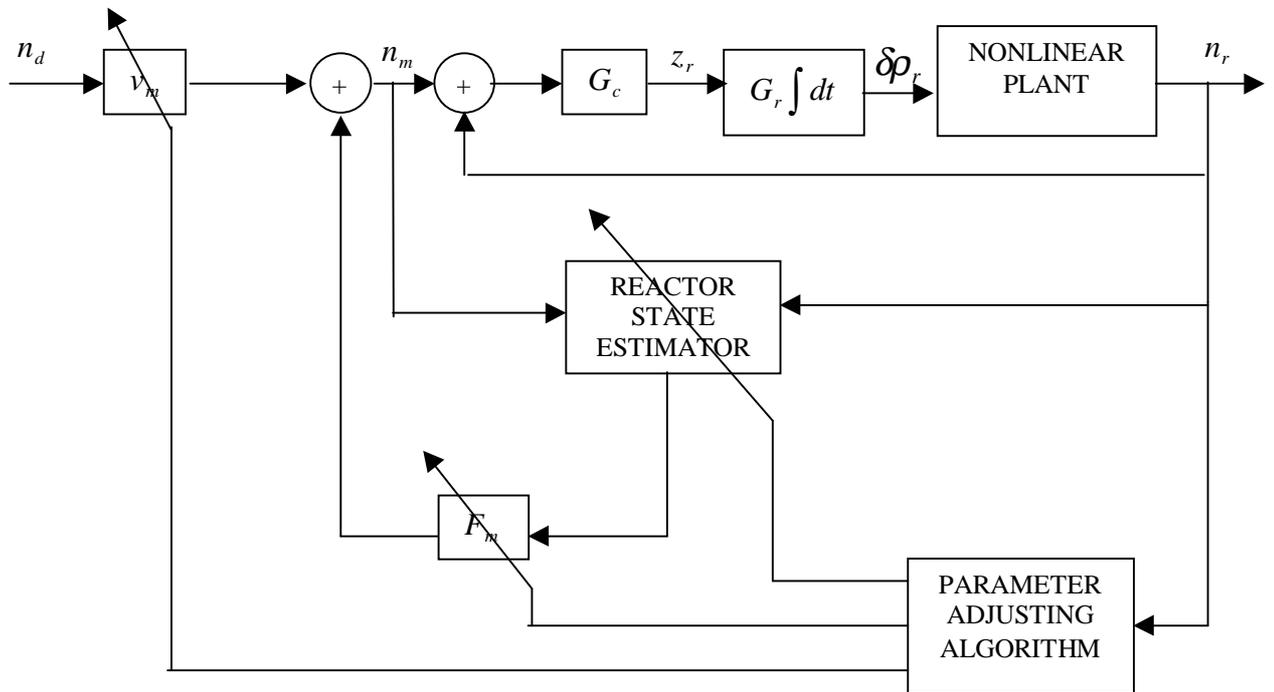
Fig. 3. Robust Optimal Self-Tuning Regulator configuration.
