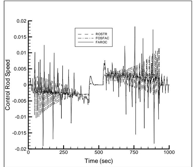
Fig. 12. Control rod speed for start-up/shut-down operation 100% → 10% → 100%.
