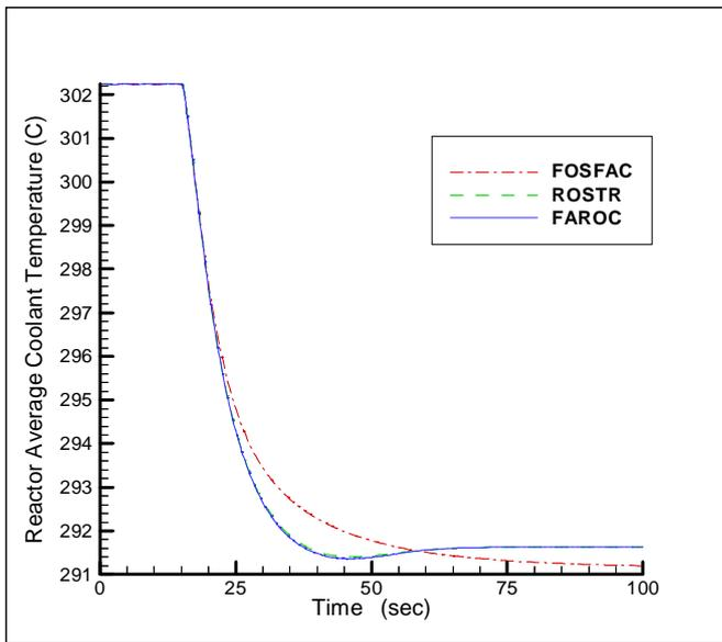
Fig. 9. Reactor average coolant temperature for 100% to 10% power level change
