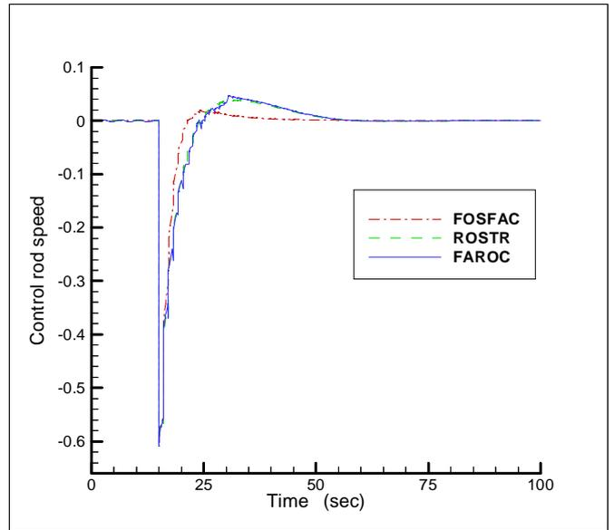
Fig. 8. Control rod speed for 100% to 10% power level change.
