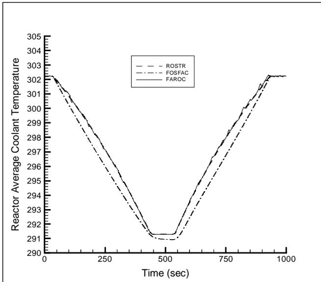
Fig. 13. Reactor average coolant temperature for start-up/shut-down operation 100% → 10% → 100%.
