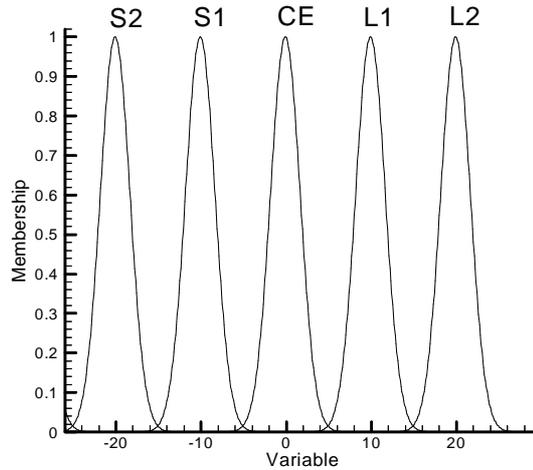
Fig. 6. Schematic of membership functions
