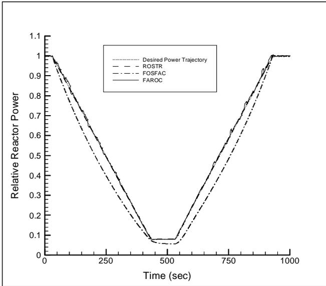
Fig. 11. Relative reactor power for start-up/shut-down operation 100% → 10% → 100%.
