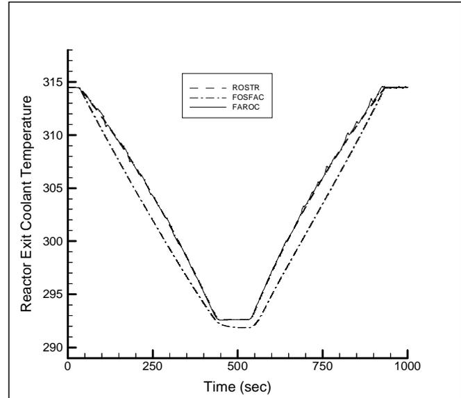
Fig. 14. Reactor exit coolant temperature for start-up/shut-down operation 100% → 10% → 100%.
