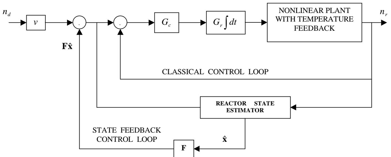
Fig. 2. State Feedback Assisted Classical Control configuration.
