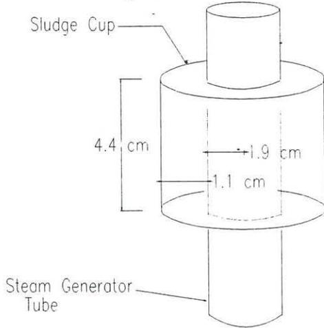
**Figure 1. Steam Generator Tube With Sludge Cup**
