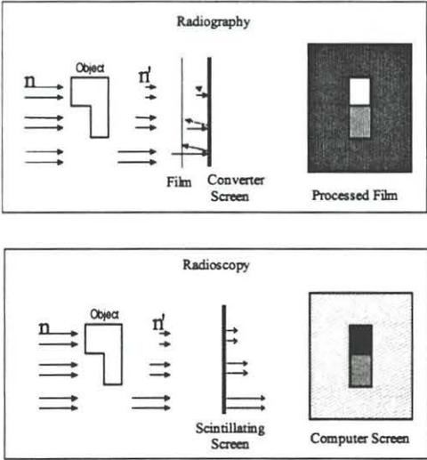
**Figure 3 – Radiography and Radioscopy Image Formation**
