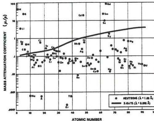
Figure 1 - Mass Attenuation Coefficients as a Function of Atomic Number<sup>1</sup>
