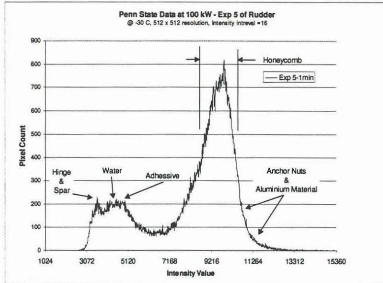
**Figure 10 -Histogram of Exposure 5 from Penn State at 100 kW<sub>t</sub>**
