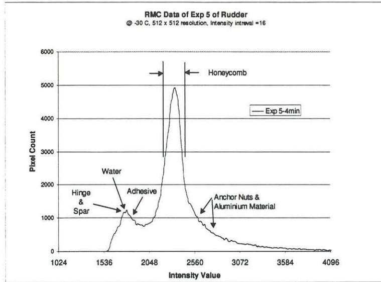
**Figure 8 - Histogram of Exposure 5 from RMC (10 kW<sub>t</sub>)**
