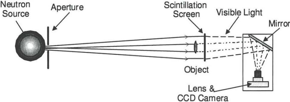
**Figure 2 - Neutron Radiography Configuration**
