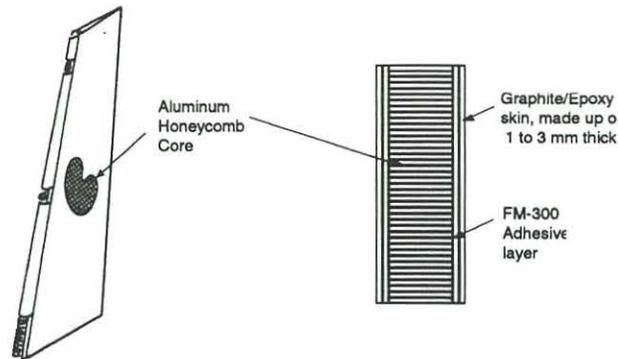
**Figure 5 - Construction of a CF-18 Rudder**
