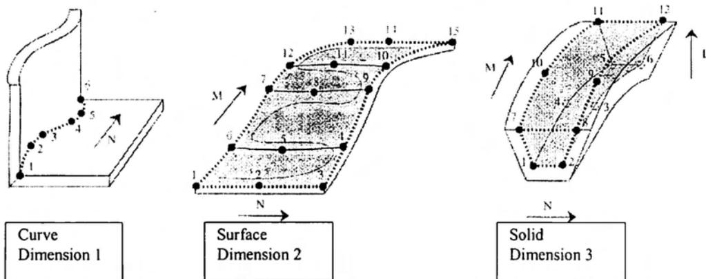
**Figure 3:** The three types of programmable work areas
