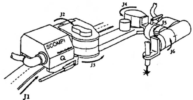
Figure 1 : The six-axis SCOMPI manipulator
