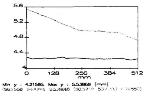
**Figure 19 :** Comparison between the original (top) and final profile of the work-piece. All units are in mm.
