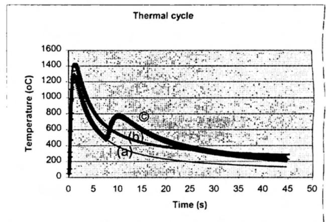
**Figure 10 :** Computed thermal cycle : (a) one wire 50°C preheat; (b) one wire 200°C preheat; (c) two wires (tandem) 50°C preheat.
