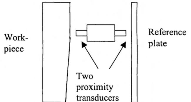
**Figure 17 :** Schematic of the sensors set-up.
