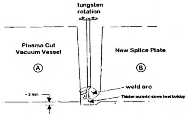
Figure 12 : The rotating tungsten electrode of the NG-TIG process. This features improves sidewalls fusion.
