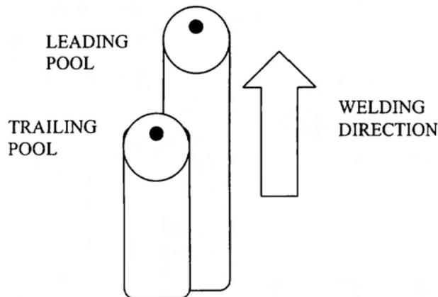
**Figure 9 :** Schematic view of the two weld pools in the SCOMPI tandem MIG process.
