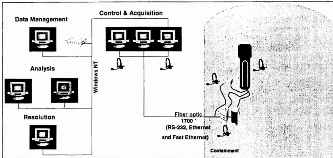
Figure 7: Gentilly II eddy current inspection set-up
