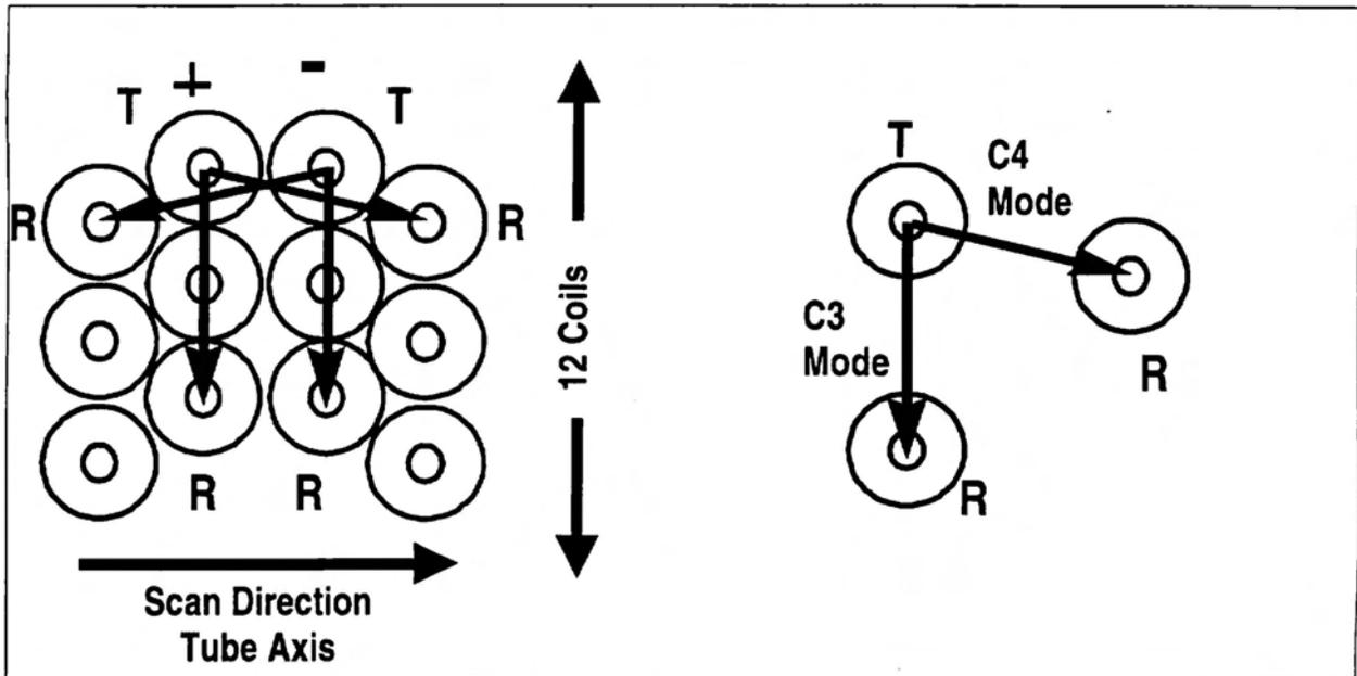
Figure 2: C6 probe coil schematics, for 13 mm diameter, Incoloy 800 tubing, showing C3 and C4 coil pairs. The C3 units are primarily sensitive to circumferential oriented cracks and the C4 units are primarily sensitive to axially oriented cracks.
