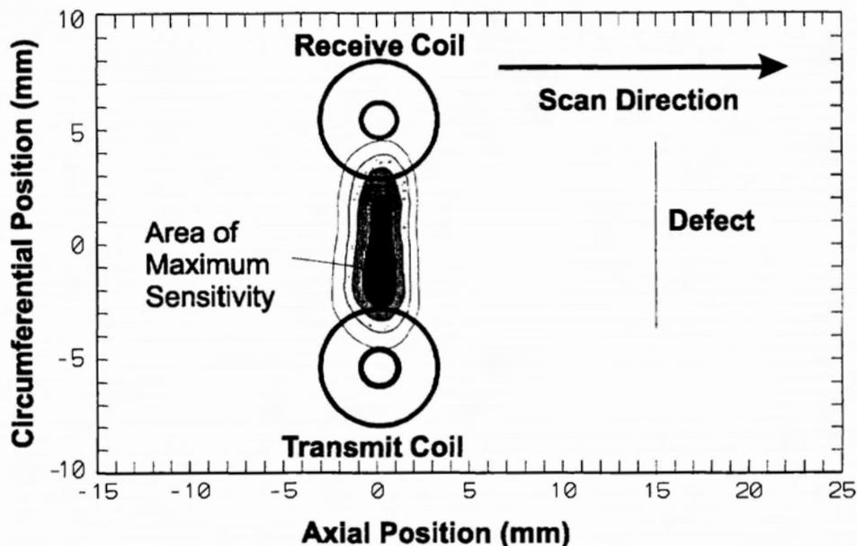
Figure 1: Computer simulation illustrating areas of sensitivity and directional properties of T/R probes.
