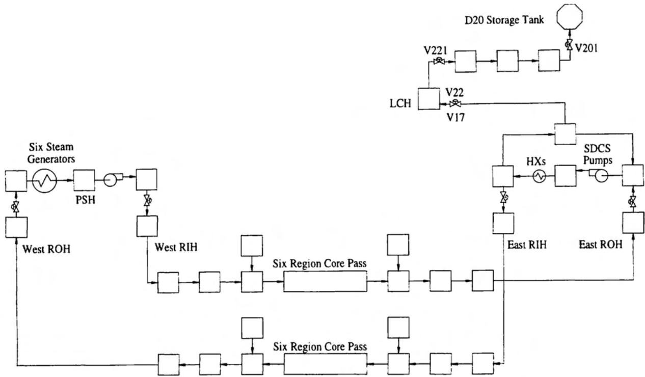
Figure 2. Sketch of the HTS model used in this assessment.
