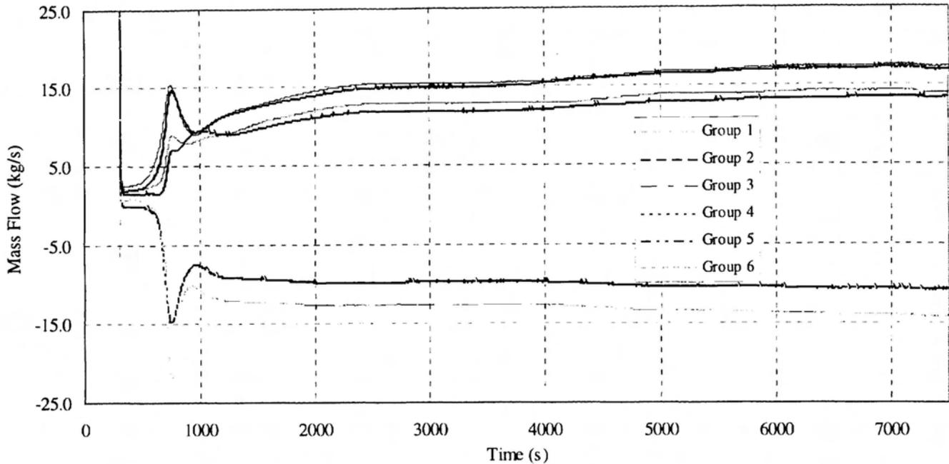
Figure 4. Typical flow distribution in the fuel channels.
