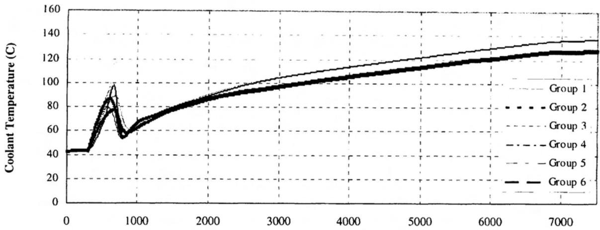
Figure 3(a). Fuel channel coolant temperature for Case 1.
