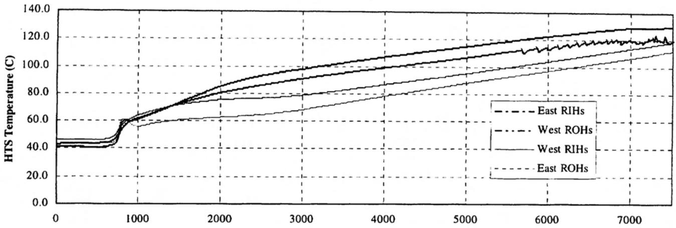
Figure 5(a). HTS temperature for Case 1.
