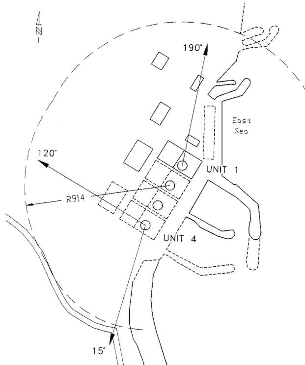
**Figure 2** Plan-view of the reactor complex showing test wind directions and release locations. The dashed line shows the 914 m (1000 yard) exclusion area boundary.
