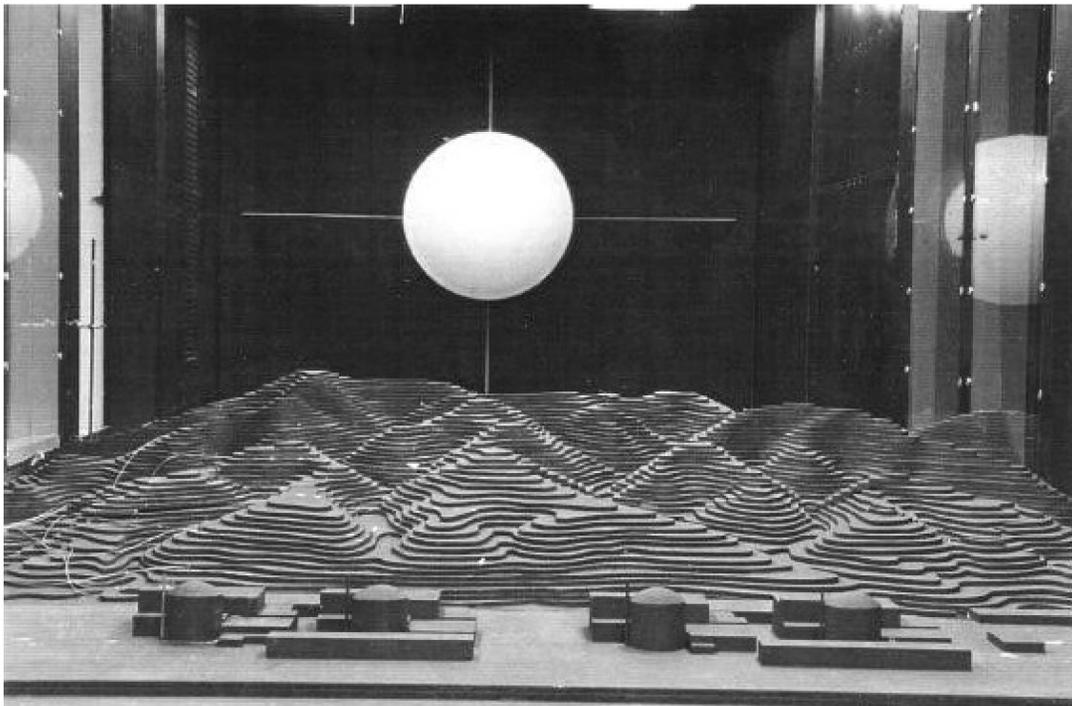
Figure 1. The wind tunnel model of the Wolsong reactor complex and the hills to the west (Hangan et al. 1997).
