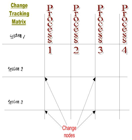
In this matrix, the process owner would obtain change data, by process, across systems, whereas the operator could obtain data by system, across processes. This dictates how we need to capture, and track our Plant Status data, such that we can sort in both planes.
