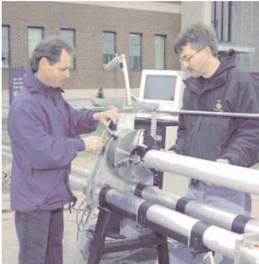
Figure 2: Loading a pipe into the PCM for monitoring
