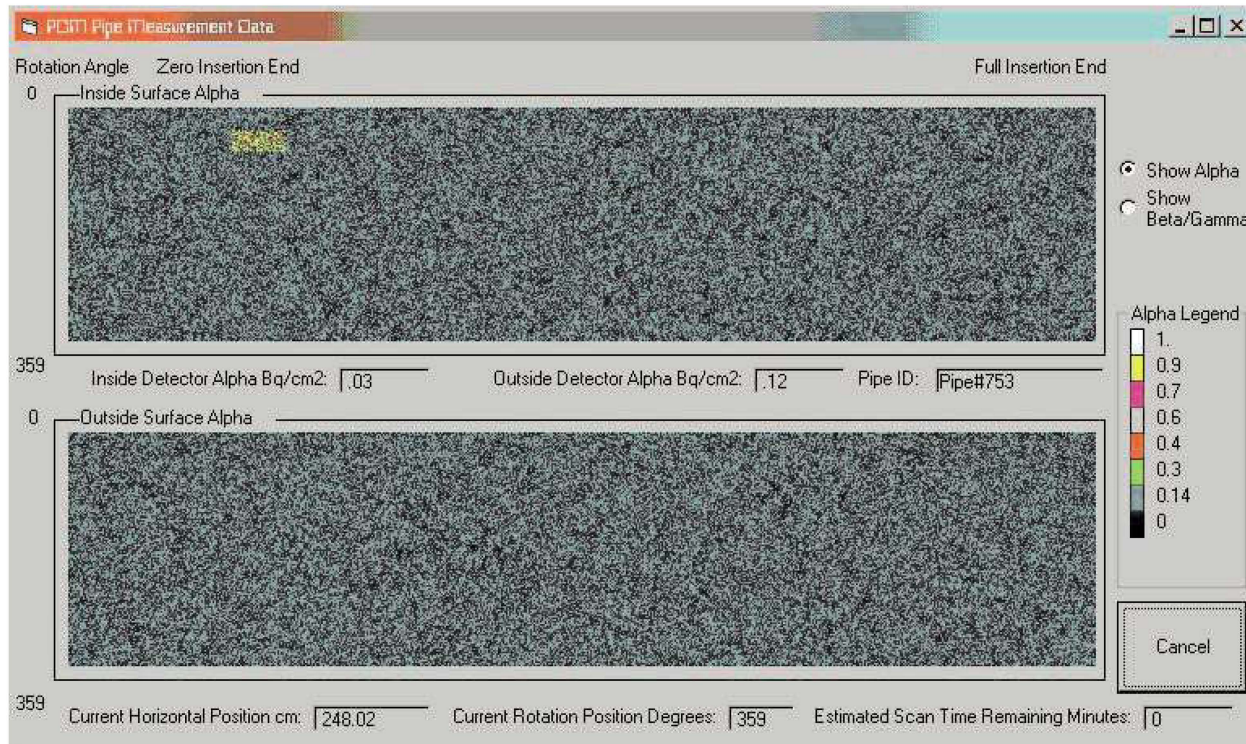
Figure 7: Graphic representation of the radioactive topography of the pipe surface
