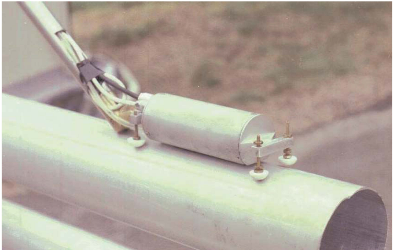
Figure 4: The external detector head riding on the top of the pipe being inspected
