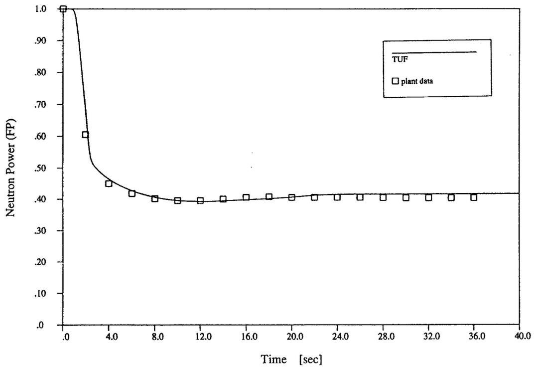
Figure 2. Comparison of neutron power transient with plant data
