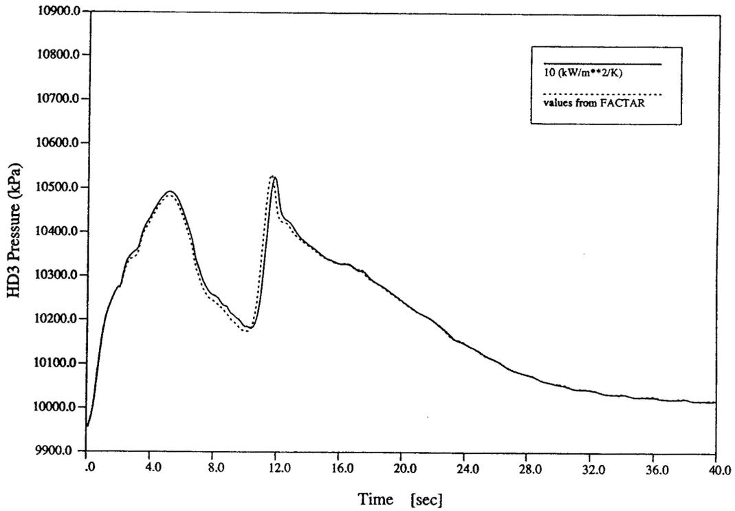
Figure 9. Comparison of HD3 pressure transients with different gap heat transfer coefficients
