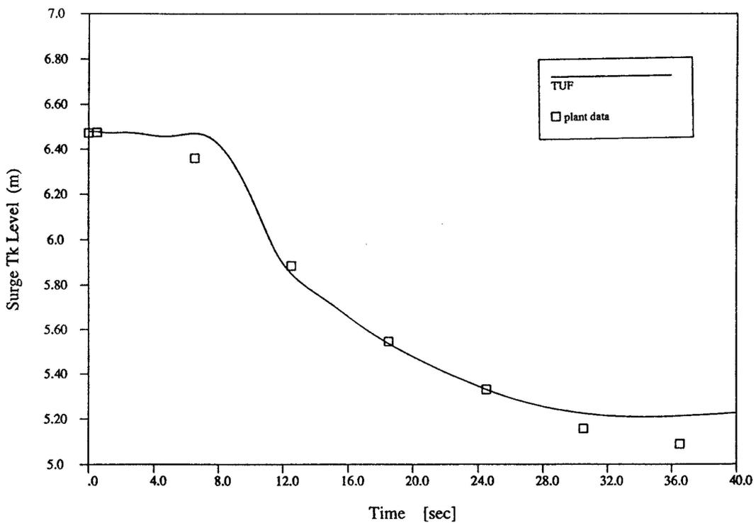
Figure 4. Comparisons of pressure and water level transients at pressurizer with plant data
