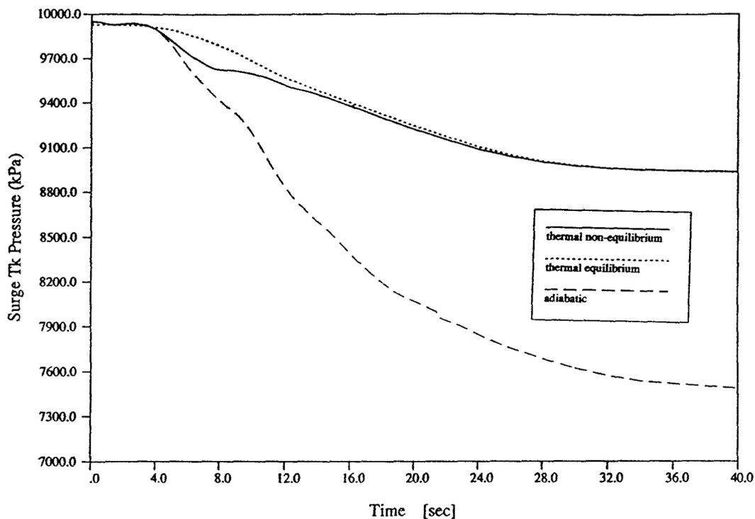
Figure 10. Comparison of pressurizer pressure transients with different models
