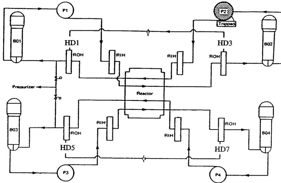
Figure 1. Location of tripped pump in the PHT circuit
