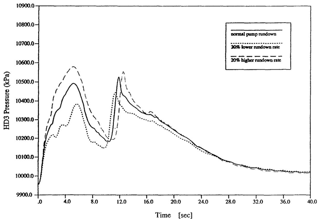
Figure 7. Comparison of HD3 pressure transients with different pump rundown rates
