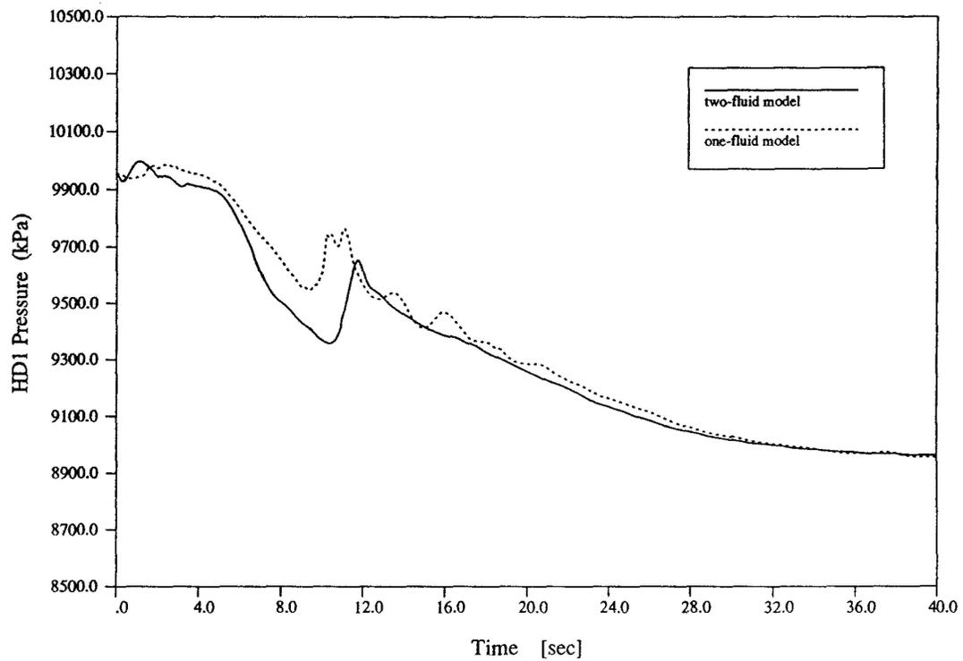
Figure 13. Comparison of HD1 pressure transients between one-fluid and two-fluid models
