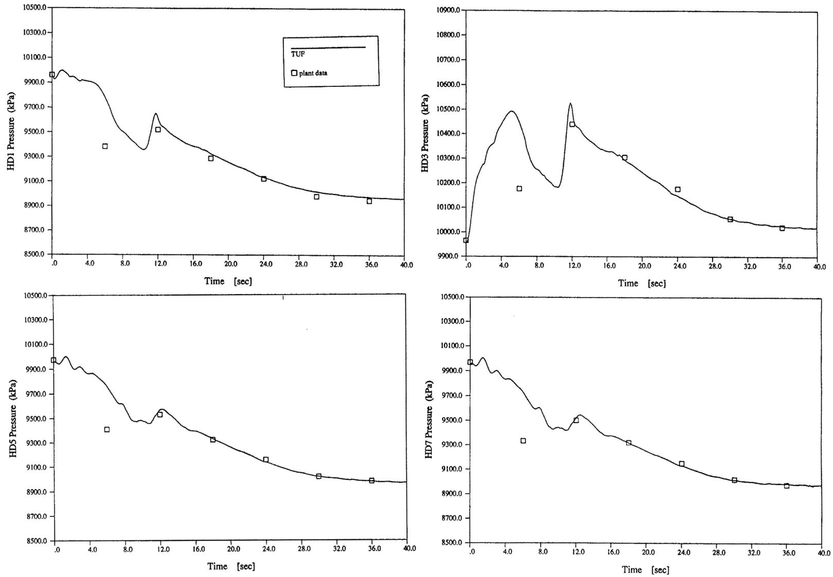
Figure 3. Comparisons of pressure transients at reactor outlet headers with plant data
