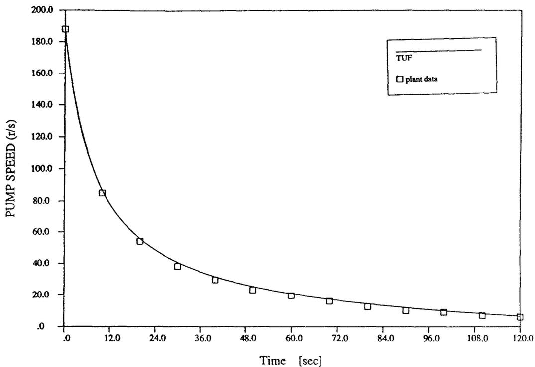
Figure 6. Comparison of pump speed with data from Darlington four pumps trip test
