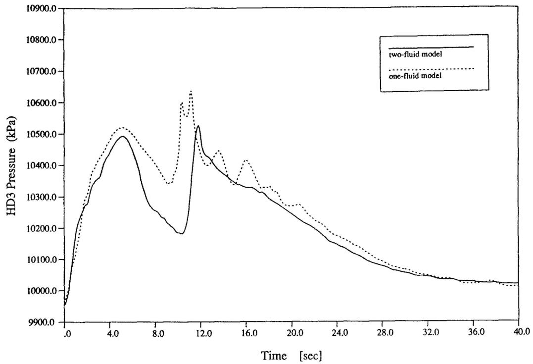
Figure 12. Comparison of HD3 pressure transients between one-fluid and two-fluid models
