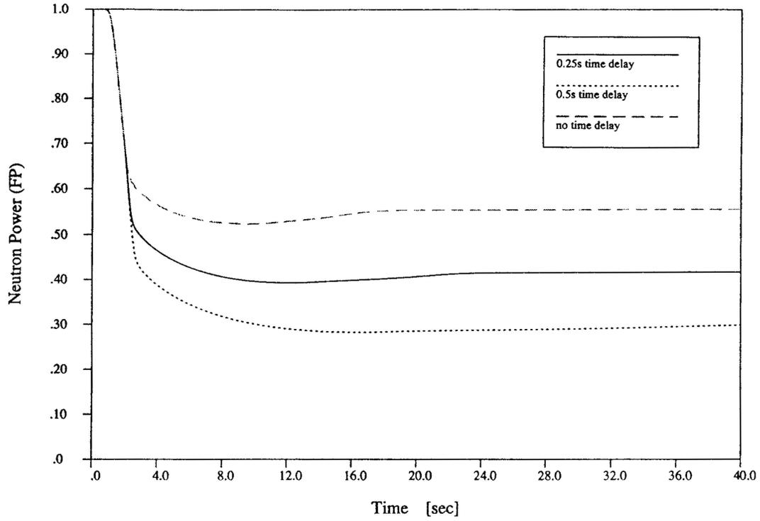
Figure 8. Comparison of neutron power transients with different actions in clutch closing
