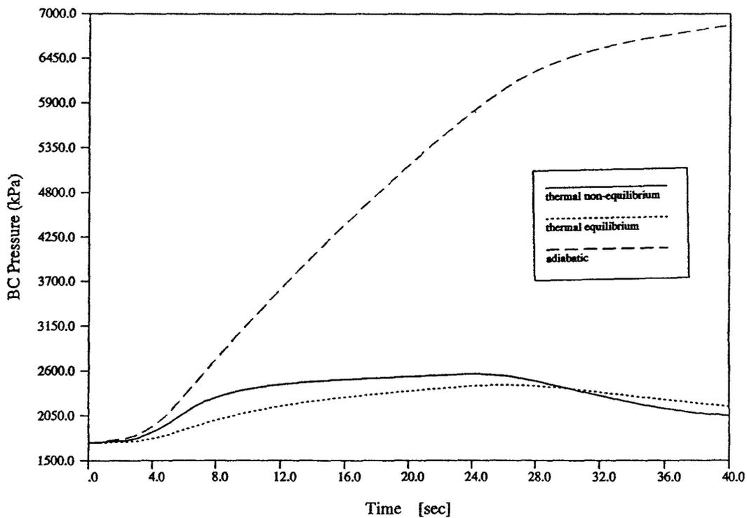
Figure 11. Comparison of bleed condenser pressure transients with different models
