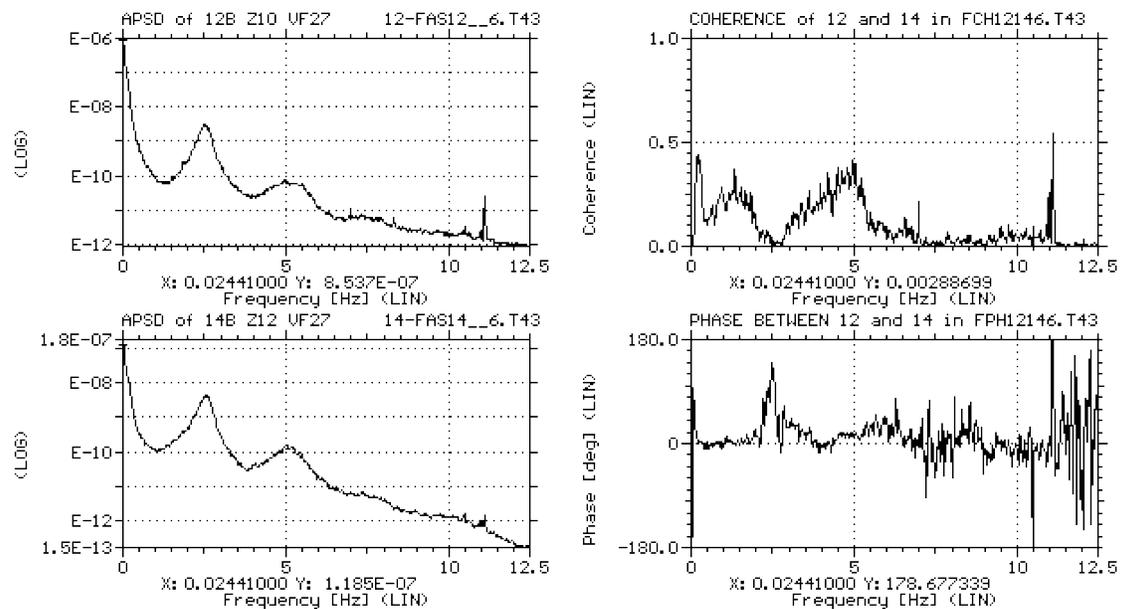
Figure 7. APSD spectra, Coherence and Phase functions of ICFD signals 12B and 14B in VFD27 measured in Unit 4 in 1999
