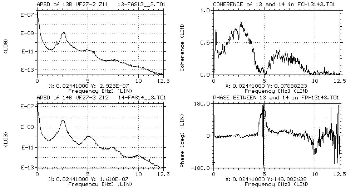
Figure 6. APSD spectra, Coherence and Phase functions of ICFD signals 13B and 14B in VFD27 measured in Unit 4 in 1996
