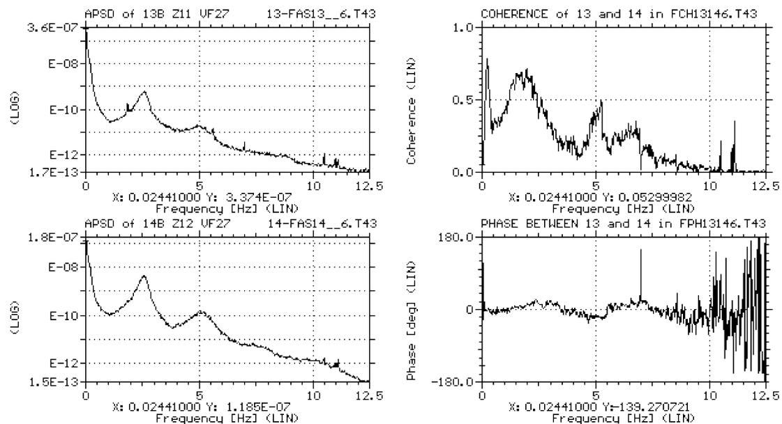
Figure 8. APSD spectra, Coherence and Phase functions of ICFD signals 13B and 14B in VFD27 measured in Unit 4 in 1999
