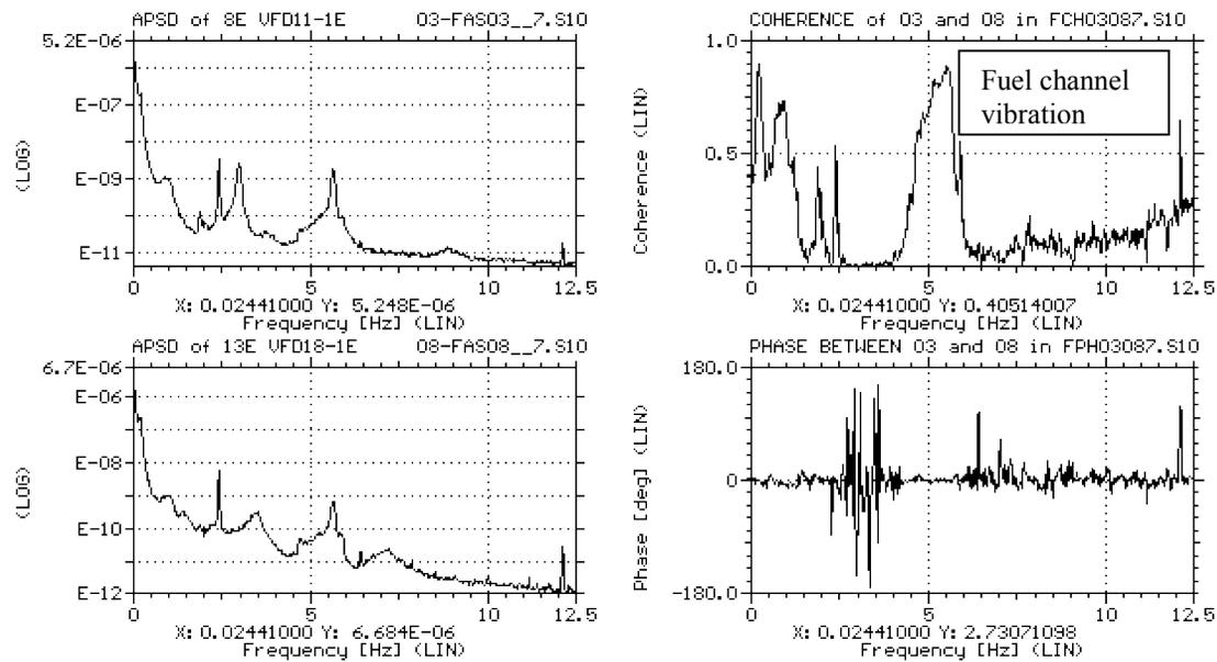
Figure 13. APSD spectra, Coherence and Phase functions of noise signals of two SDS1-E ICFDs VFD11-1E and VFD18-1E lined up along the same set of fuel channels in Zones 6 and 8 in Darlington Unit 3.
