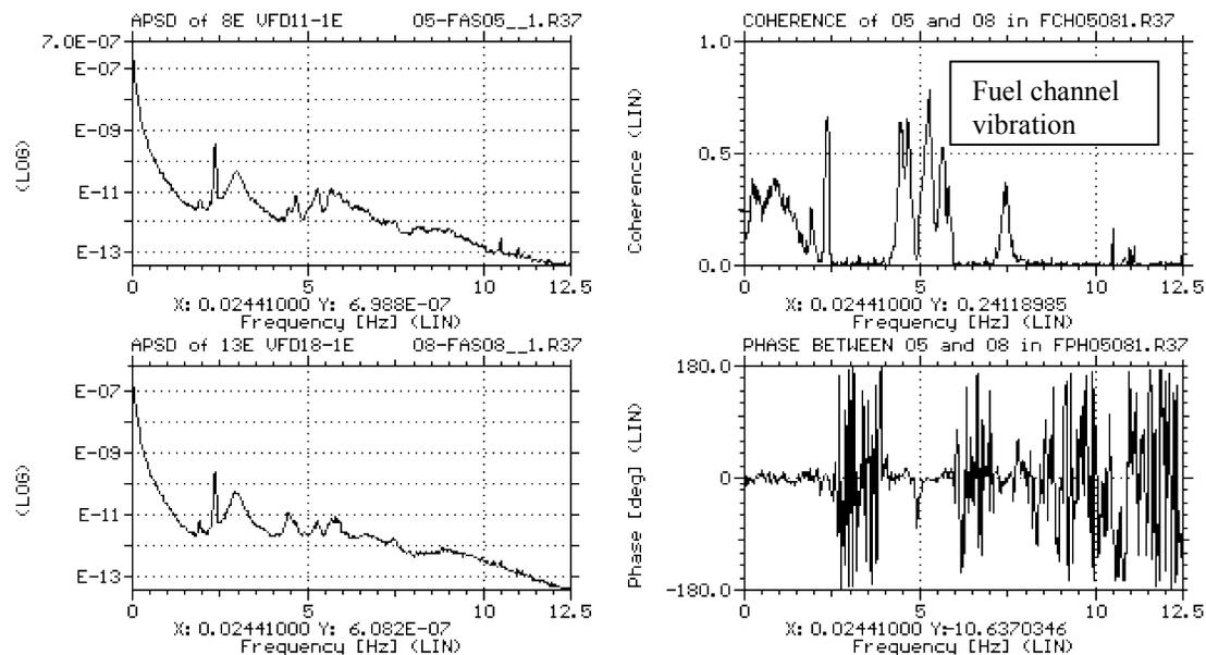
Figure 12. APSD spectra, Coherence and Phase functions of noise signals of two SDS1-E ICFDs VFD11-1E and VFD18-1E lined up along the same set of fuel channels in Zones 6 and 8 in Darlington Unit 2.
