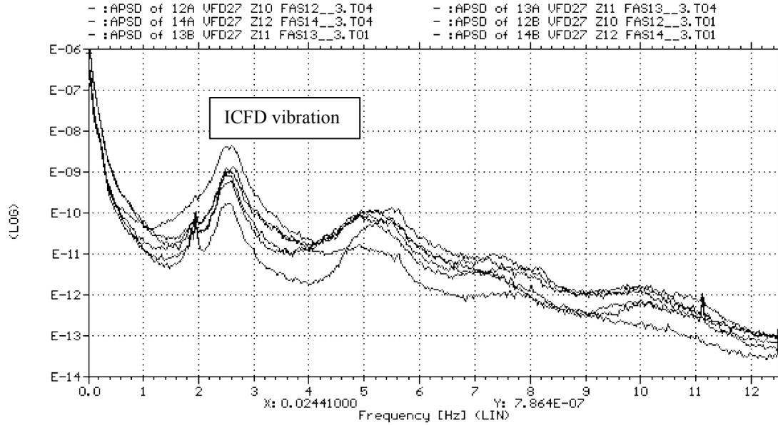
Figure 3. APSD spectra of ICFD signals in VFD27 measured in Unit 4 in 1996.
