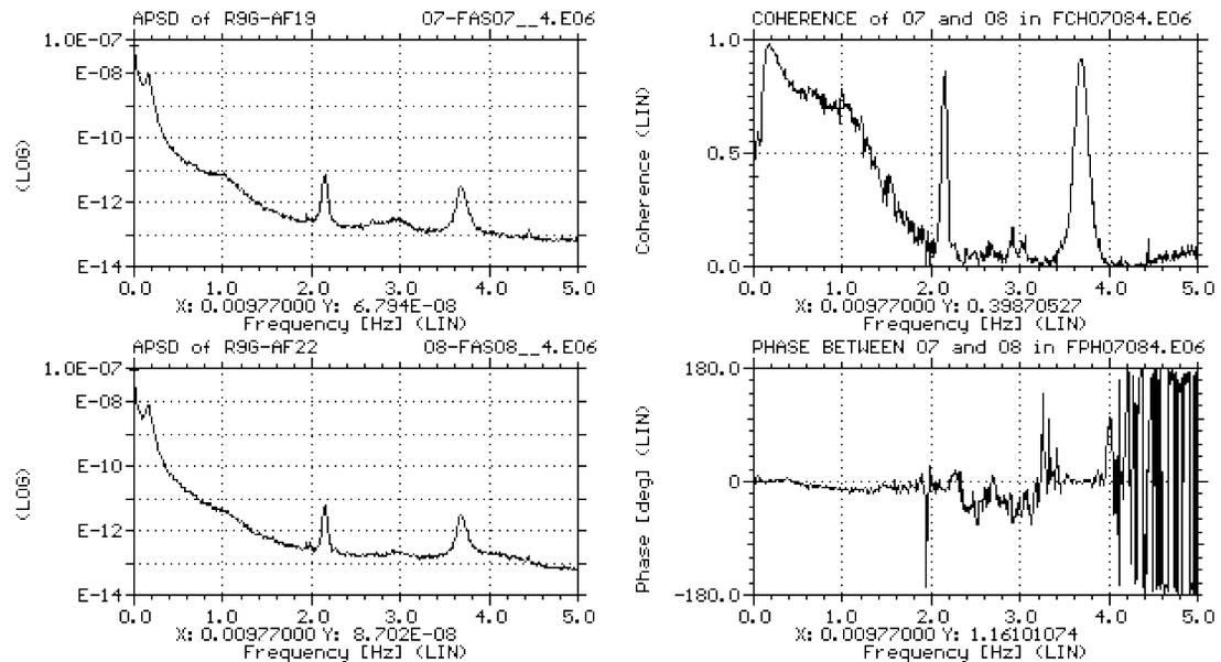
Figure 10. APSD spectra, Coherence and Phase functions of noise signals of two SDS2-G ICFDs located in the same horizontal detector tube, HFD9, measured in Pickering-B Unit 5.
