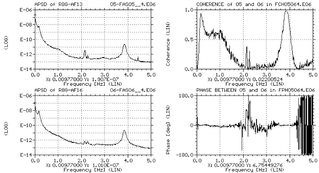
Figure 9. APSD spectra, Coherence and Phase functions of noise signals of two SDS2-G ICFDs located in the same horizontal detector tube, HFD8, measured in Pickering-B Unit 5.
