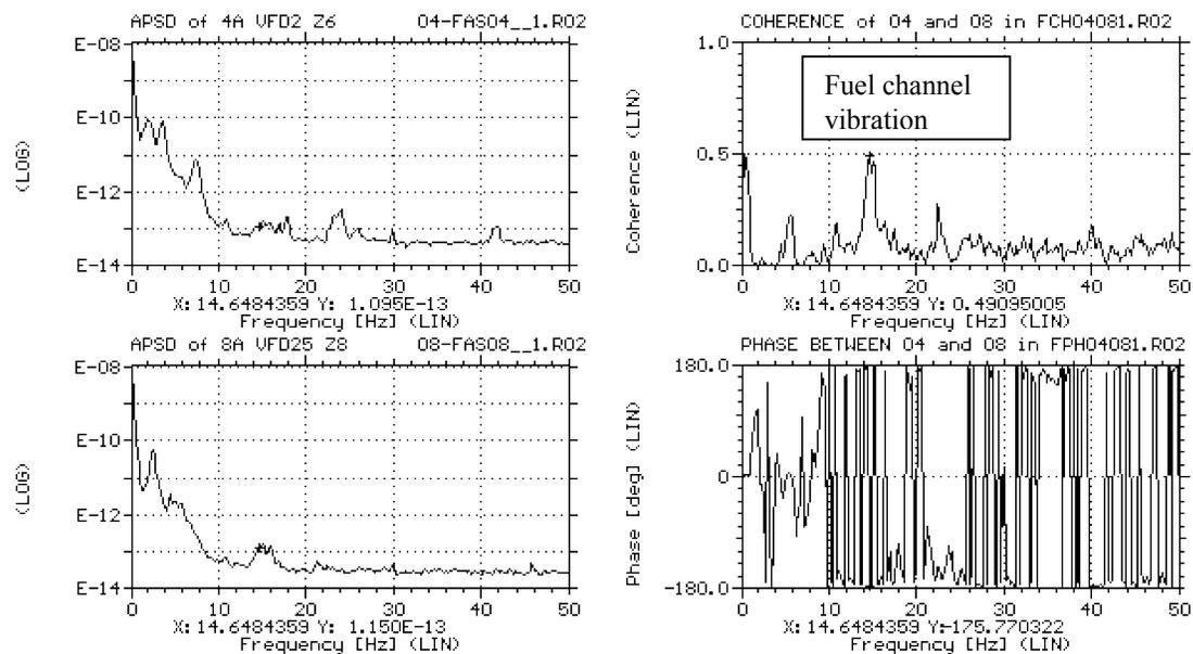
Figure 16. APSD spectra, Coherence and Phase functions of noise signals of RRS-A ICFDs in Zones 6 and 8, lined up along the same set of fuel channels in Darlington **Unit 2**.
