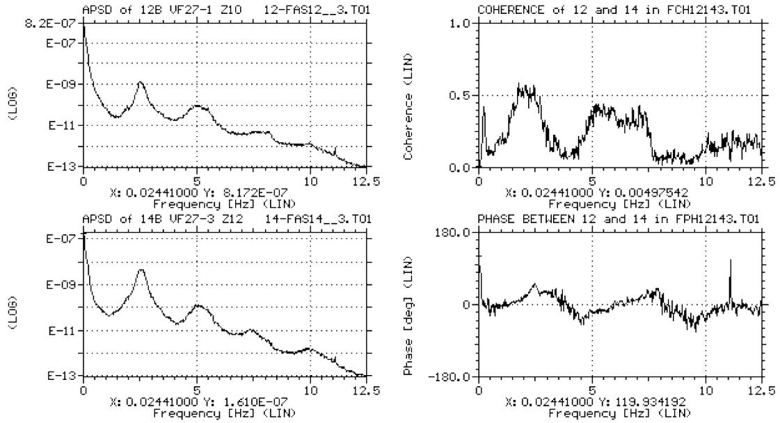
Figure 5. APSD spectra, Coherence and Phase functions of ICFD signals 12B and 14B in VFD27 measured in Unit 4 in 1996.
