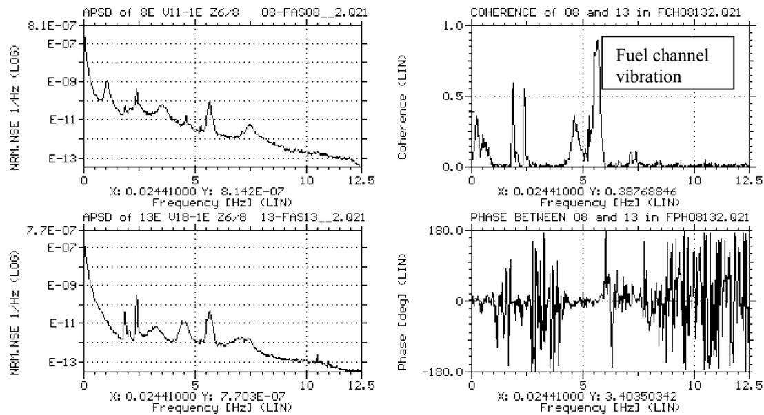
Figure 11. APSD spectra, Coherence and Phase functions of noise signals of two SDS1-E ICFDs VFD11-1E and VFD18-1E lined up along the same set of fuel channels in Zones 6 and 8 in Darlington Unit 1.
