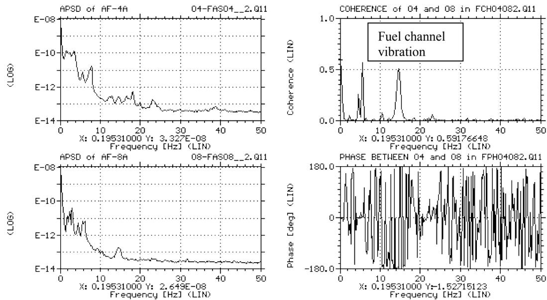
Figure 15. APSD spectra, Coherence and Phase functions of noise signals of RRS-A ICFDs in Zones 6 and 8, lined up along the same set of fuel channels in Darlington **Unit 1**.
