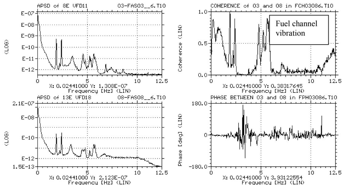
Figure 14. APSD spectra, Coherence and Phase functions of noise signals of two SDS1-E ICFDs VFD11-1E and VFD18-1E lined up along the same set of fuel channels in Zones 6 and 8 in Darlington Unit 4.
