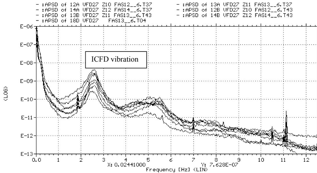
Figure 4. APSD spectra of ICFD signals in VFD27 measured in Unit 4 in 1999
