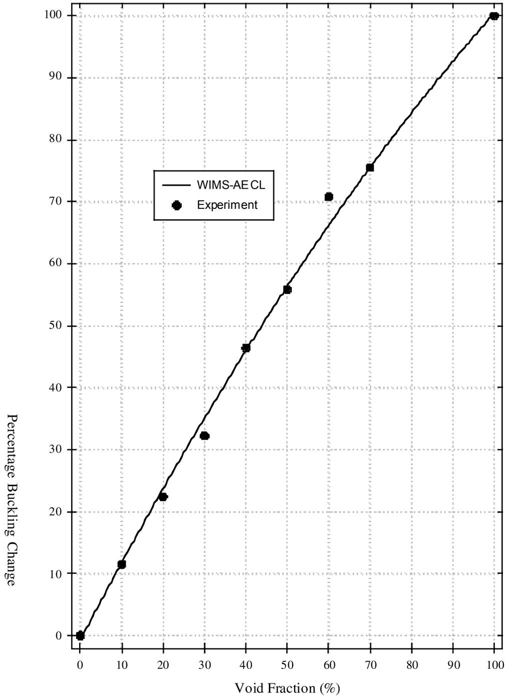
Figure 3: Buckling change with void fraction
