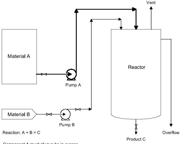
Component A must always be in excess of component B to avoid an explosion
