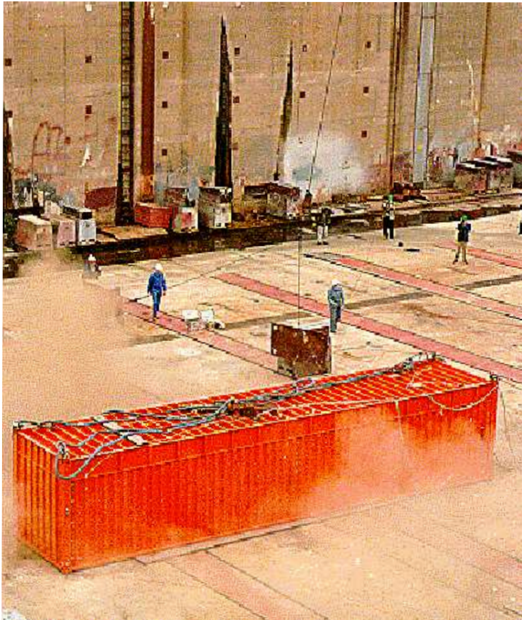
Figure 5. The picture shows the container shortly after hitting the drop test unyielding foundation
