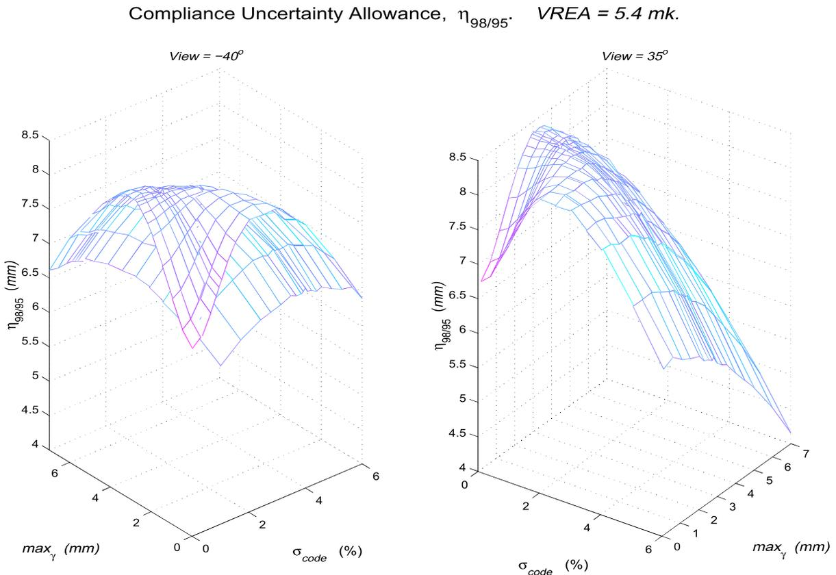
Fig. 5. Relationship between the *compliance uncertainty*, the code error and the gap measurement error.
