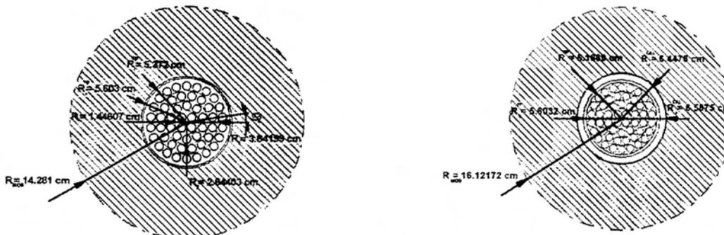
FIGURE 17: AVERAGE CELL FOR CNA NPP (A), AND FOR CNE NPP (B)
