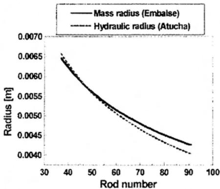
FIGURE 5: CURVE WITH THE "MASS" AND "HYDRAULIC" RADIUS OF CANDU AND ATUCHA.
