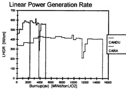
FIGURE 10: AVERAGED POWER HISTORY FOR A CANDU FUEL ROD AND CARA FUEL IN CANDU NPP.
