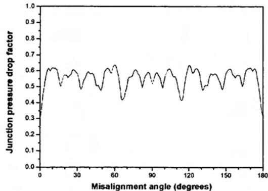
FIGURE 15: CALCULATED END PLATE FRICTION FACTOR COEFFICIENT FOR CARA FUEL USING THE DEVELOPED MODEL.
