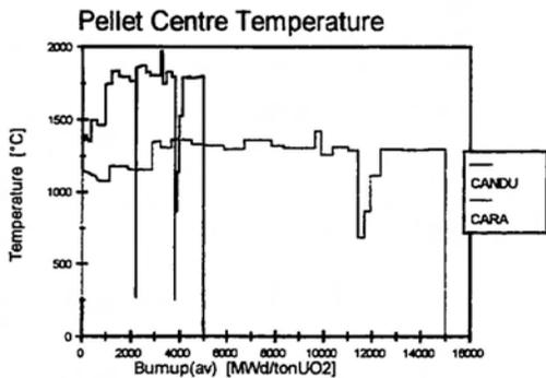
FIGURE 11: AVERAGED TEMPERATURE AT THE PELLET CENTER OF A CANDU FUEL ROD CARA FUEL.
