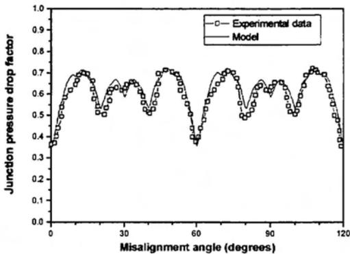
FIGURE 14: COMPARISON OF CANDU END PLATE FRICTION FACTOR COEFFICIENT BETWEEN EXPERIMENTAL AND THE DEVELOPED MODEL.
