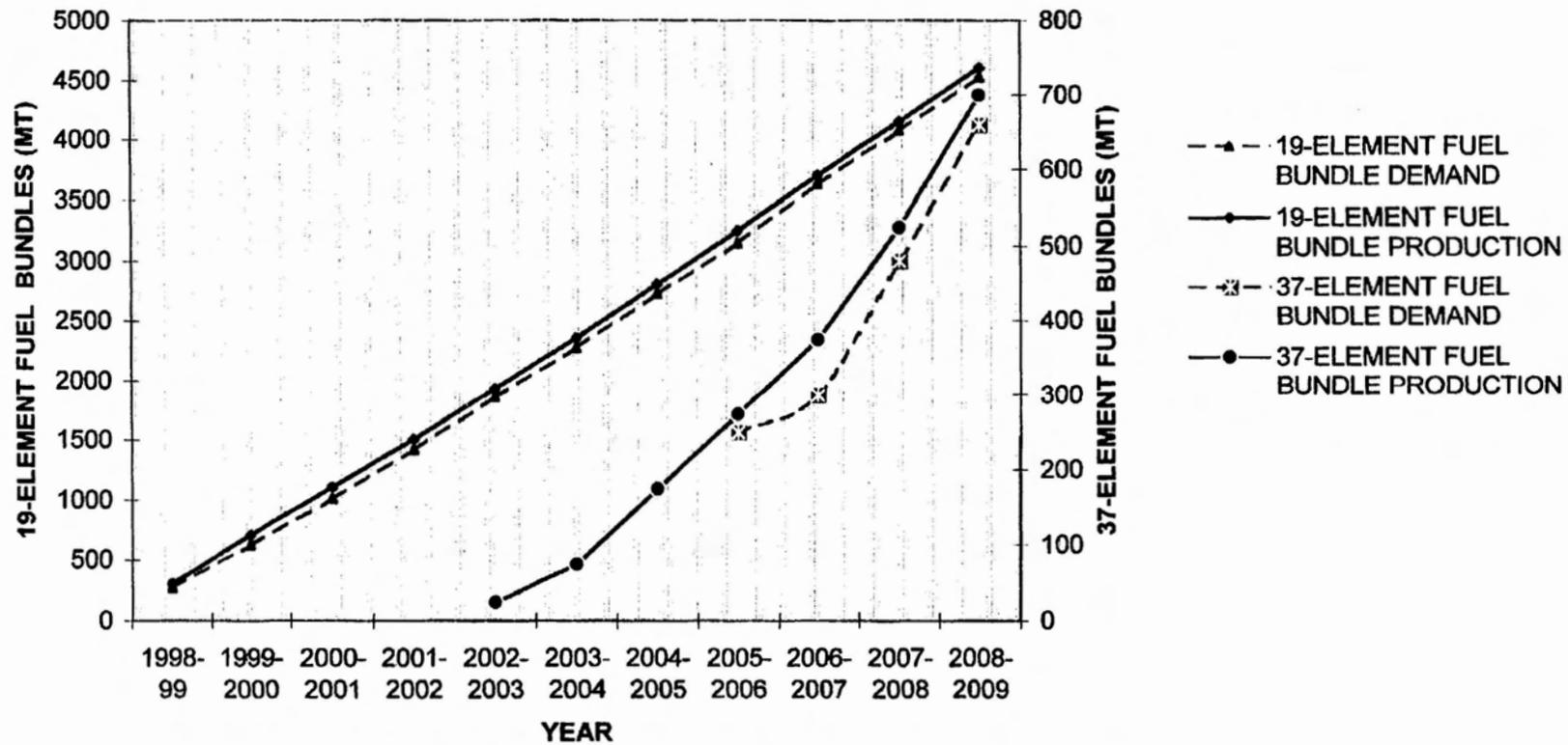
**FIG.2: CUMULATIVE DEMAND AND PRODUCTION OF PHWR-220 MWe AND PHWR-500 MWe FUELS IN INDIA**
