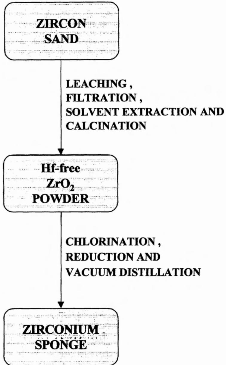
**FIG.3: PROCESS STEPS FOLLOWED IN NFC FOR THE PRODUCTION OF NUCLEAR GRADE ZIRCONIUM SPONGE FROM ZIRCON SAND**
