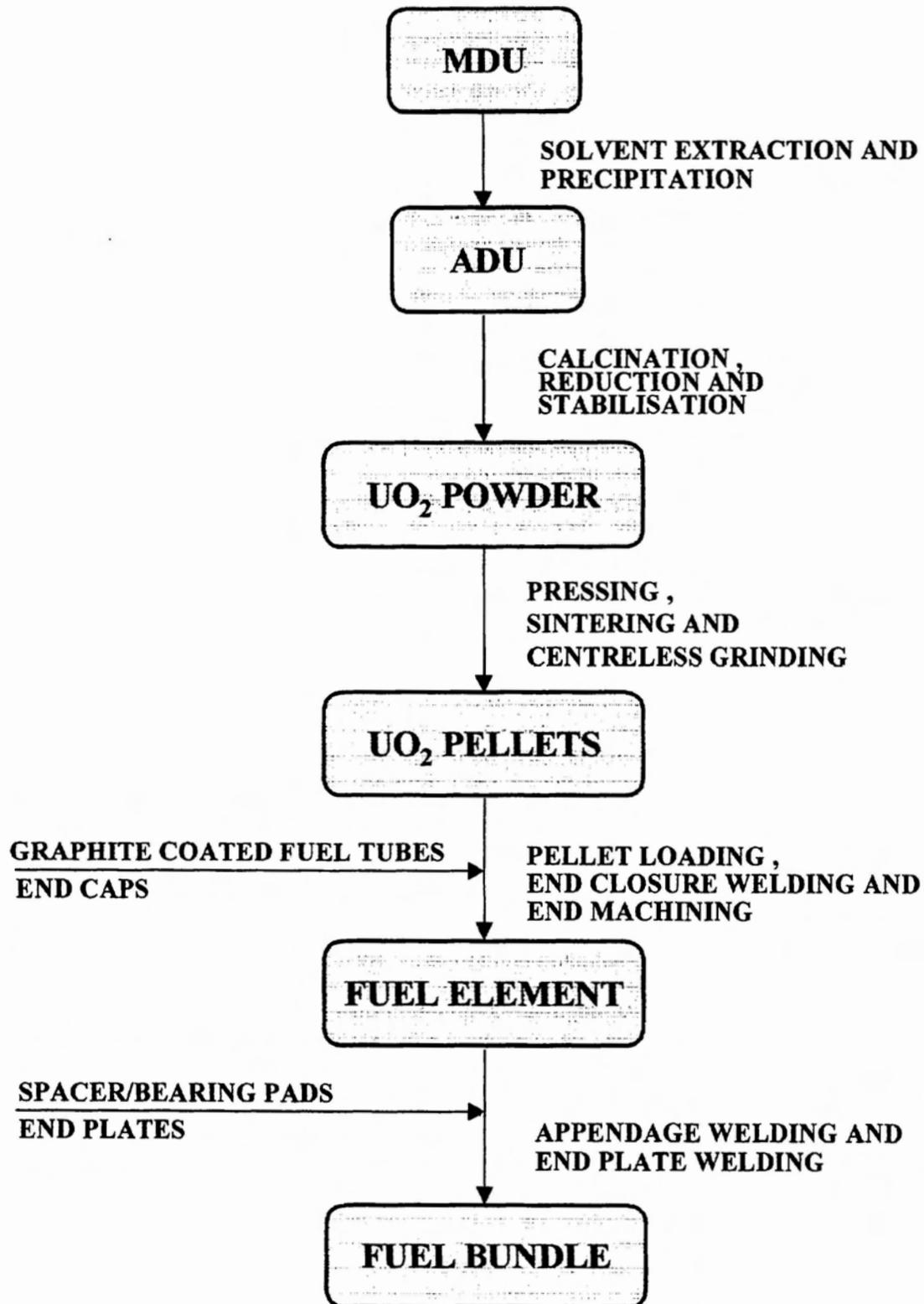
**FIG.5: PROCESS FLOW SHEET FOLLOWED IN NFC FOR PHWR FUEL PRODUCTION**
