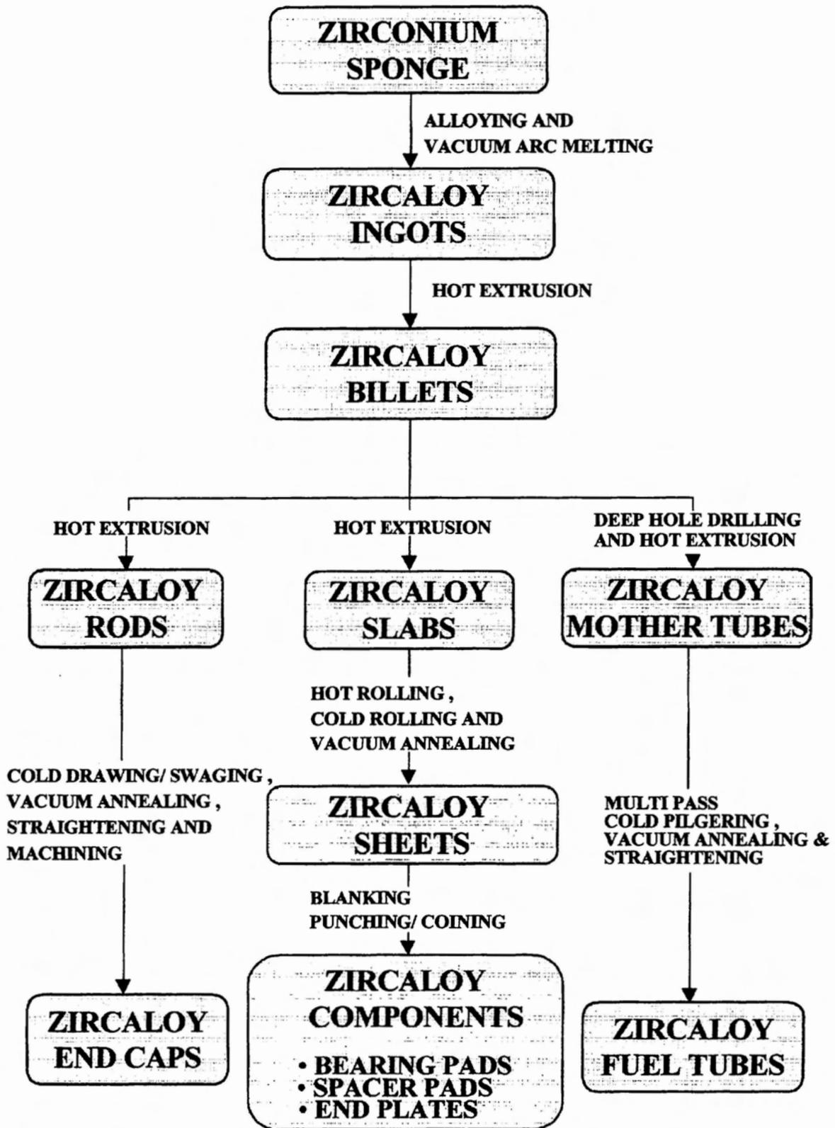
**FIG.4: PROCESS FLOW SHEET FOLLOWED IN NFC FOR THE PRODUCTION OF ZIRCALOY-4 FUEL TUBES AND COMPONENTS**
