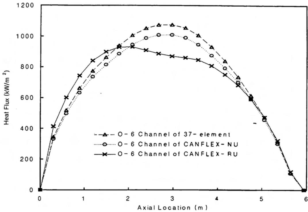
Fig. 3. Local Heat Flux Distribution of O-6 Channel in CANDU-6
