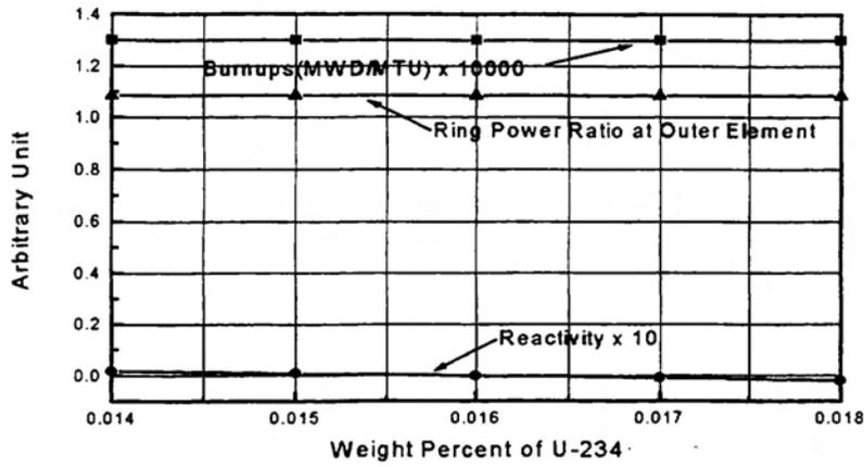
(a) Sensitivity of  $^{234}\text{U}$  on Lattice Characteristics
