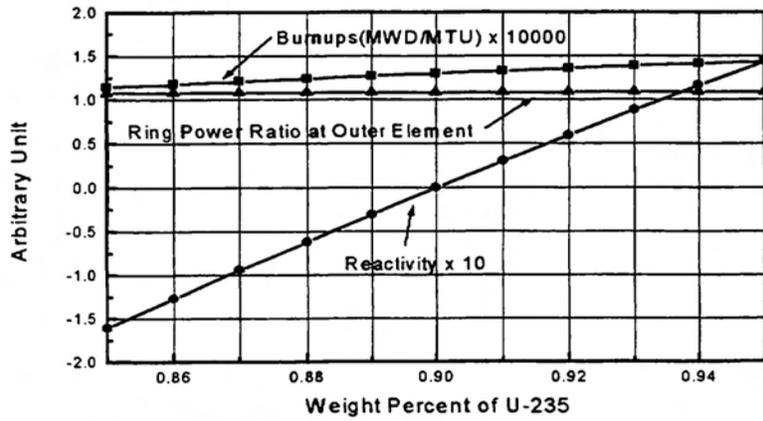
(b) Sensitivity of  $^{235}\text{U}$  on Lattice Characteristics
