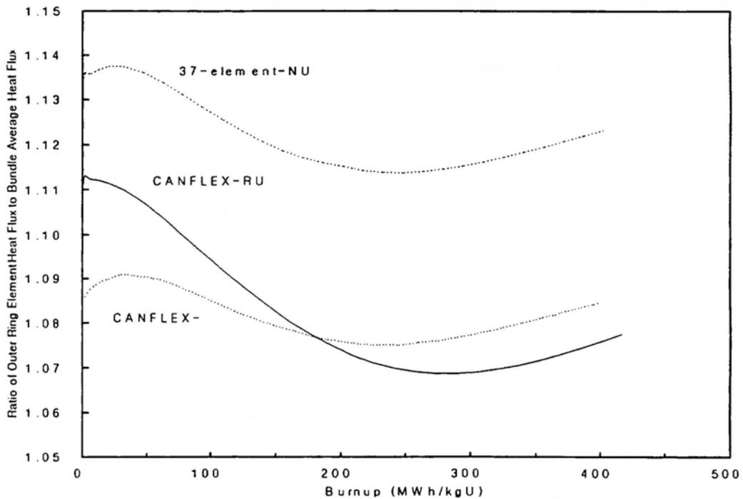
Fig. 4. The Behavior of BRFF(Bundle Radial Form Factor) with respect to Bundle Burnup
