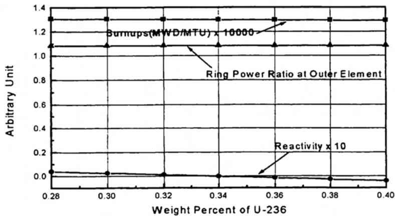
(c) Sensitivity of  $^{236}\text{U}$  on Lattice Characteristics
