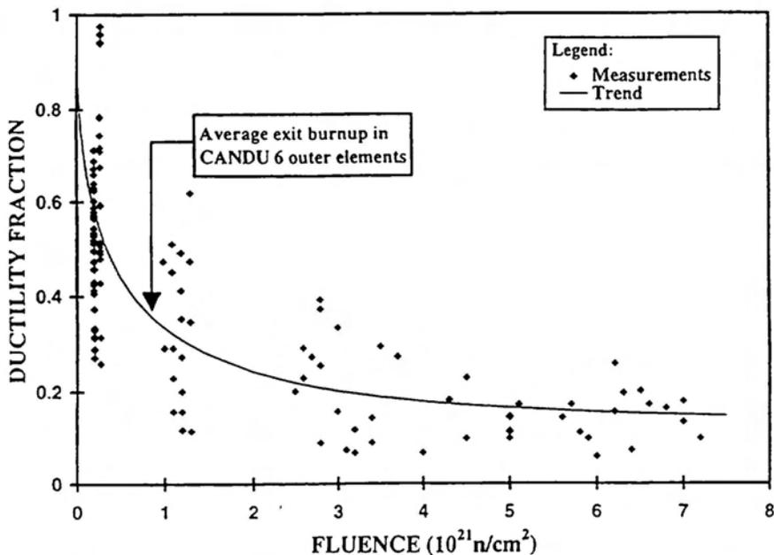
(b) Effect of Neutron Damage
