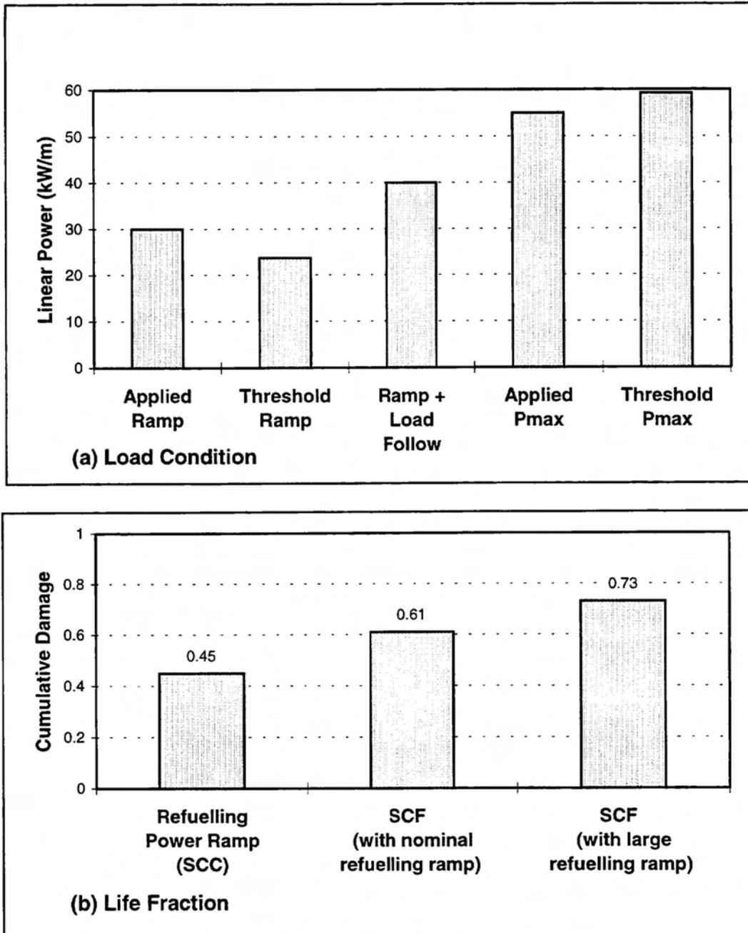
Figure 6: Fatigue Life of Bruce Fuel: Weekly Cycles
