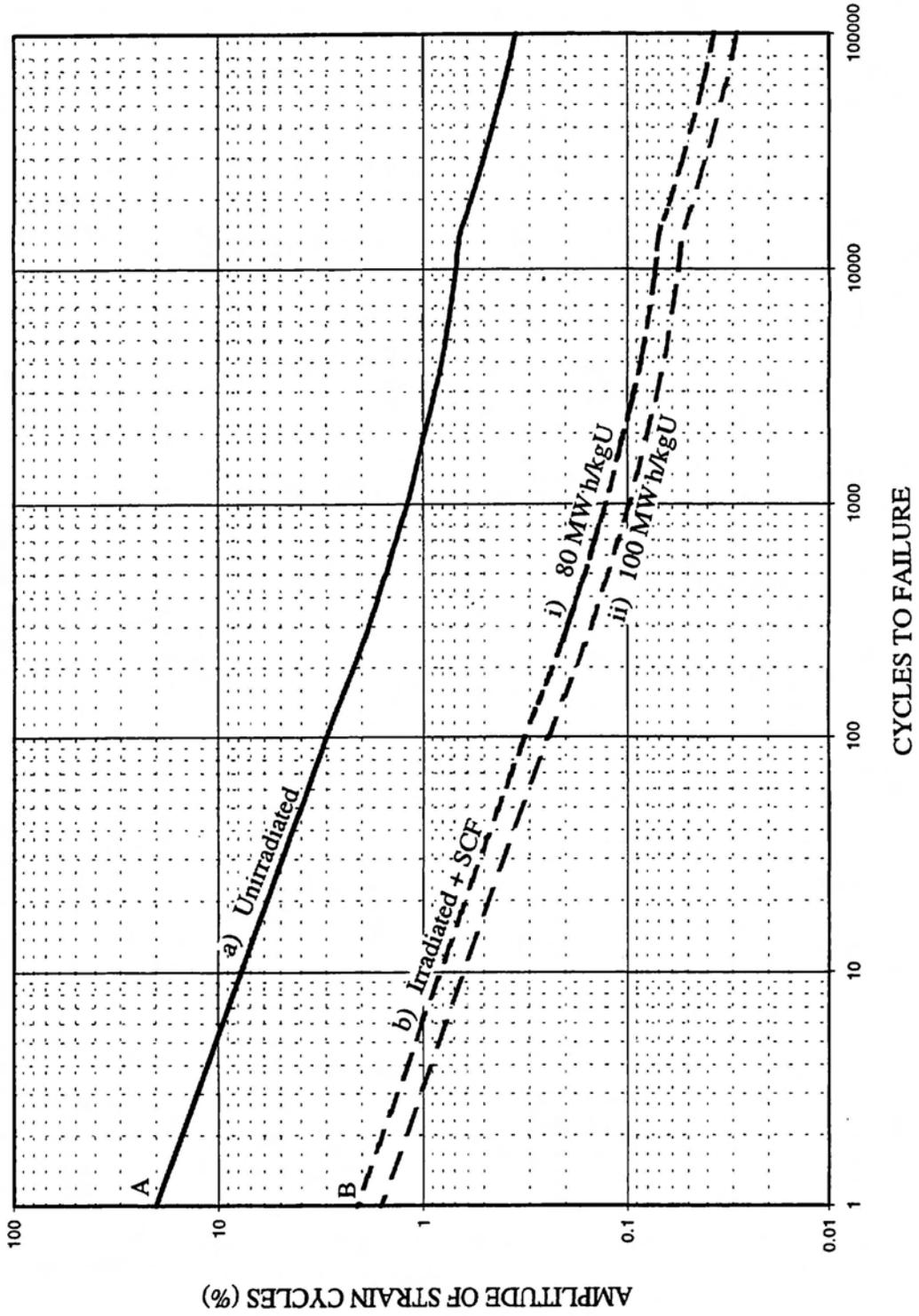
Figure 3: Effect of Corrosive Environment and Irradiation on the Fatigue Life of Zircaloy
