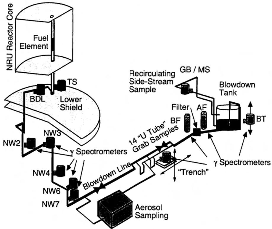
Figure 1: Schematic Drawing of the Blowdown Test Facility
